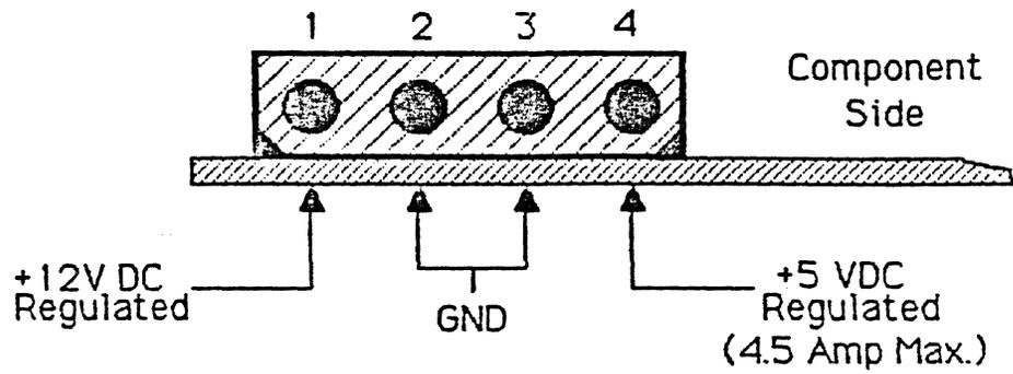
Note: Current requirements for the +12 Volt DC supply depend on the serial adapter board used.
