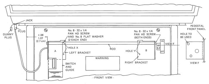
Installation of Optional Front Paper Low Switch Kit
