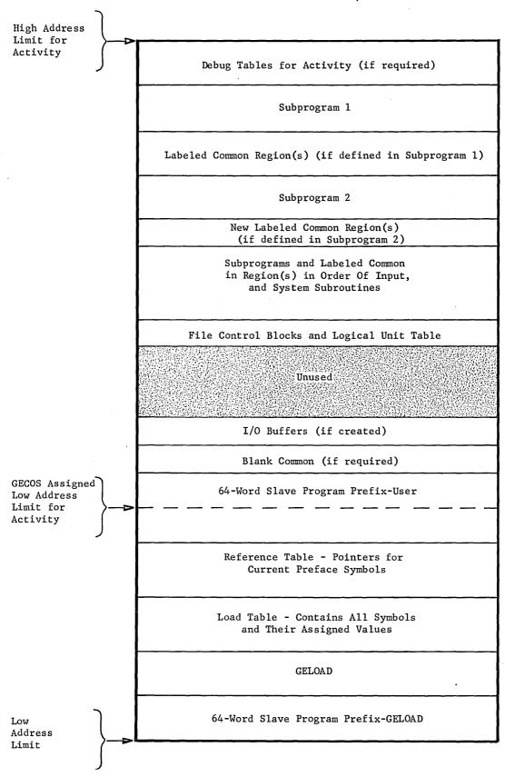
Figure 1. High-Loaded Memory Layout for Relocatable Subprograms
