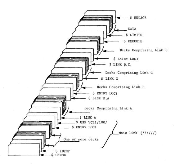
Figure 5. Deck Setup For A Linked Program
