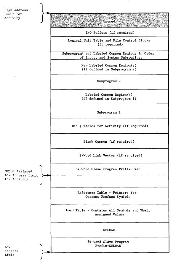
Figure 2. Low-Loaded Memory Layout for Relocatable Subprograms
