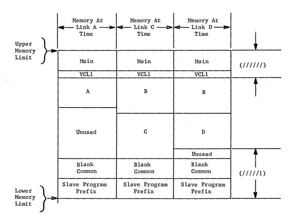
Figure 6. Memory Layout Resulting From Loading Linked Program Of Figure 5.
