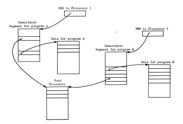
Figure 24. Common Pure Procedure Used Concurrently by Two Processors in Dual Configuration.
