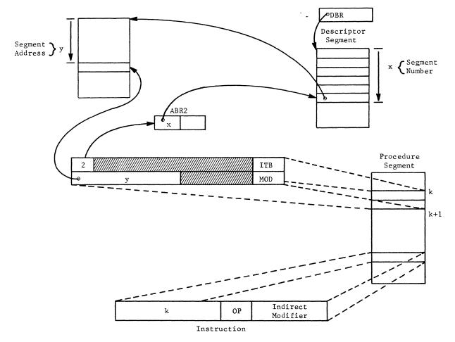
Figure 20. An ITB Pair is Used to Refer to Another Segment
