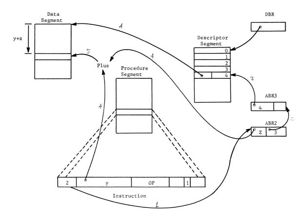
Figure 21. Operation of a Base Pair
