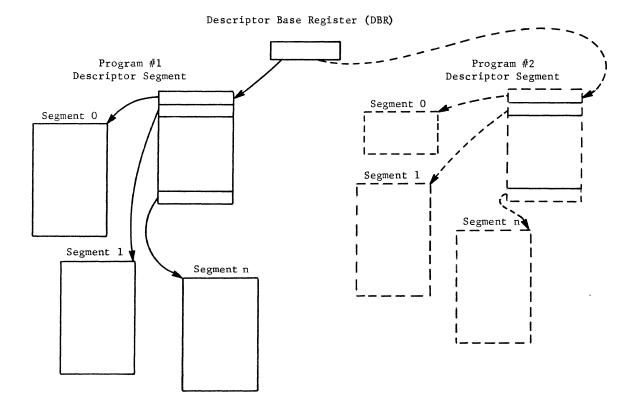
Figure 15. The DBR Determines which Segments the Processor May Access
