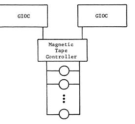
Figure 4. Single-Channel Peripherals Connected to a GIOC
