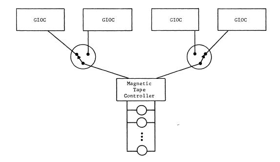
Figure 7. Two Peripheral Switches and Four GIOC's
