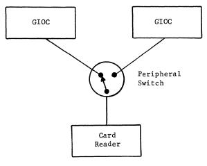
Figure 6. A Peripheral Switch and Two GIOC'S
