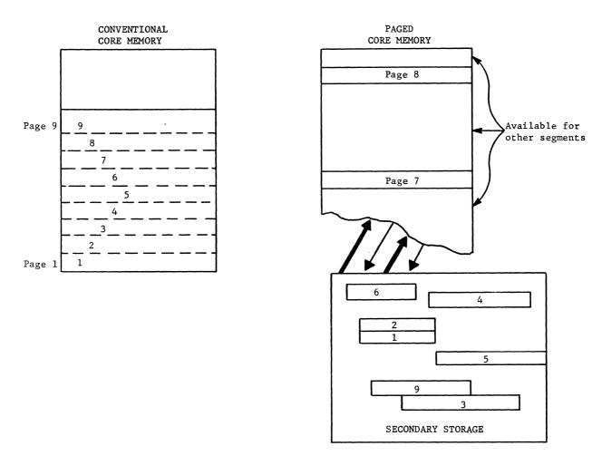
Figure 25. Frequently-Used Pages Occupy Any Available Blocks of Core Memory
