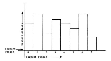
Figure 13. Two-Coordinate Addressing in the GE-645
