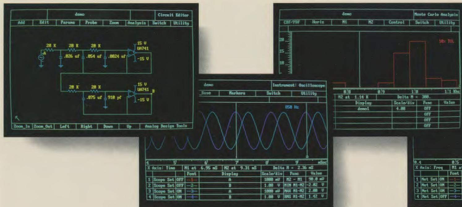
**PART OF FUTURENET'S INTEGRATED CAE ENVIRONMENT FOR PCS.** The DASH-Analog Workbench is based on what has become industry standards in CAE: Berkeley SPICE simulation software (versions 2G6 and 3) and DASH-4 Schematic Designer for fast and easy schematic capture, both running on the IBM® PC AT.
