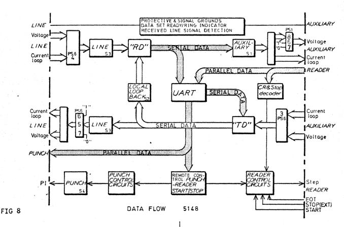
ERROR. Data must come from UART together with signal DR. DR is fed back to UART as signal DRR which resets DR. UART accepts data as long as DR=0. A delay between DR and DRR is arranged in circuit: A17:4-C1-A17:5. This is a simulated "data receive" signal. Start condition and DR activate PI. As long as start is active, every DR gives a PI and this continues until start is taken away.
