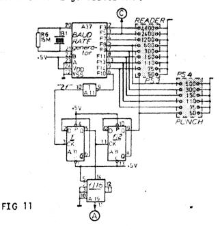
This generator is crystal controlled by B1. The generator makes it possible to get all baud rates except 50 bps directly. See table Fig. 12.
