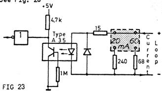
This can be set-up for different currents, 20mA or 60mA, by jumpers PS5:6,7,8,9. With no jumper it is the transmitting device that determines the current value.
