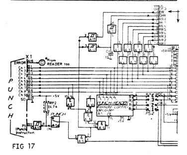
Normally DC1 - DC4 come from LINE or AUXILIARY but when the READER uses the PUNCH, DC1 and DC4 come from the tape.
