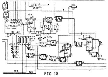
A device performing CR normally needs extra time for the operation. If the control circuits for the READER do not delay the reading a new word would be read and probably lost. The reason is the fact there is no "handshake" between the READER and the other equipment. The normal operation is to read a new word as soon as UART has transmitted the last received word (TRE).
