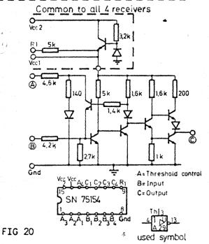
The threshold control has no logical function. It is used here for fail-safe operation by leaving the terminal open. Thus the output will go H if the input goes to O or open-circuit condition.
