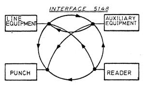
FIG 1 Different data paths possible by jumper set ups
