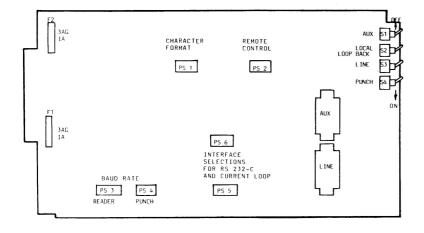
Figure 1. Facit 5148 — Localization of switches
