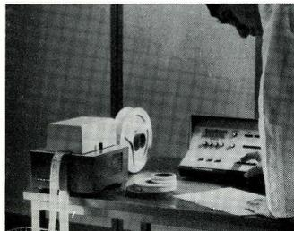
**Computer output:** processed data, programs, memory contents (during debugging for example), tapes for data transmission and for the control of machines and processes.
