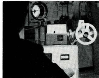
**Recording** of laboratory data and industrial measurements. Swift and simple subsequent processing is assured when values are taped.
