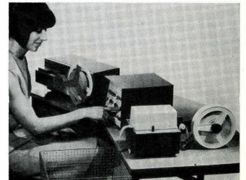
**Duplication of tapes** on special equipment, for example Facit PE 1300, which replaces worn tapes and makes conversions between various track-systems, tape materials and codes.
