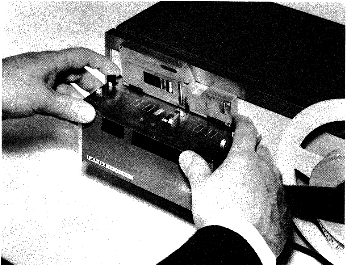
Fig. 5 - 5 Changeover to different tape width
