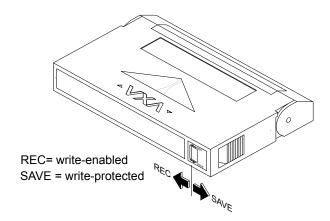
**Figure 3-3** Setting the write-protect switch
