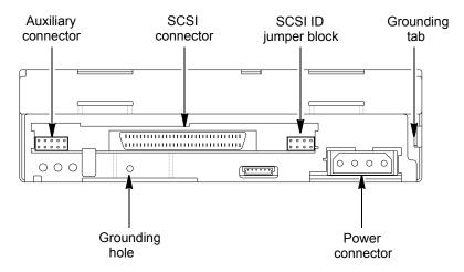
Figure 2-1 Internal SCSI drive: back-panel components
