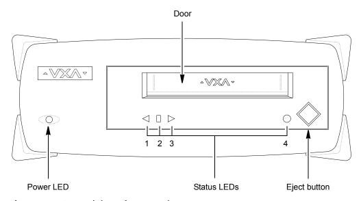
Figure 3-2 External drive: front-panel components
