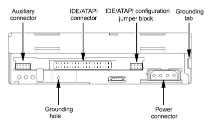
Figure 2-7 Internal IDE/ATAPI drive: back-panel components
