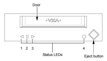
Figure 1-2 Internal drive: front-panel components
