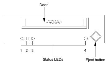
Figure 3-1 Internal drive: front-panel components
