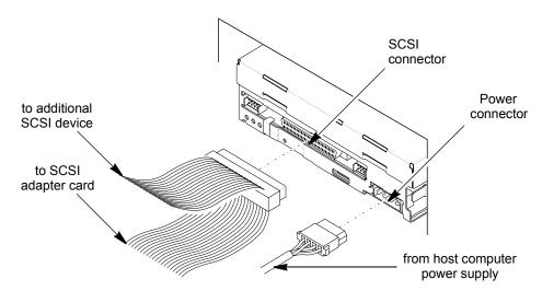
**Figure 2-4** Connecting the SCSI cable and power cable (another device is the last device on the bus)
