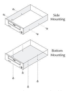
**Figure 2-10** Screw mounting configurations (internal model)
