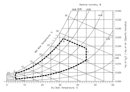
Figure 8-3 Internal drive: Operating temperature and humidity ranges
