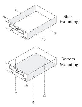
**Figure 2-6** Screw mounting configurations (internal model)
