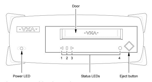
Figure 1-3 External drive: front-panel components
