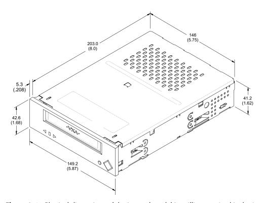
**Figure 8-1** Physical dimensions of the internal model in millimeters (and inches)
