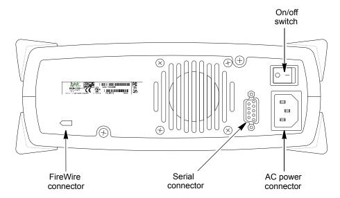
Figure 1-7 External FireWire drive: back-panel components
