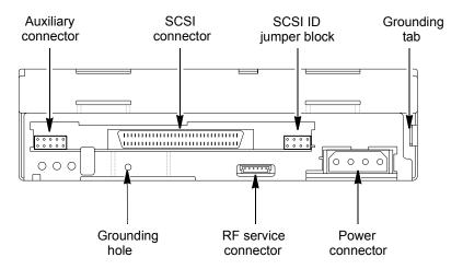
Figure 1-4 Internal SCSI drive: back-panel components
