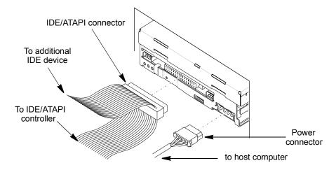
**Figure 2-9** Connecting the IDE/ATAPI cable and power cable
