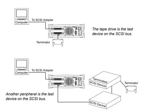
Figure 2-12 Terminating the SCSI bus for the external model
