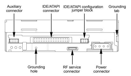
Figure 1-5 Internal IDE/ATAPI drive: back-panel components
