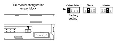
**Figure 2-8** Setting the IDE/ATAPI configuration jumper
