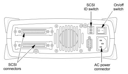
Figure 2-11 External SCSI drive: back-panel components
