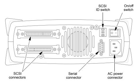
**Figure 1-6** External SCSI drive: back-panel components
