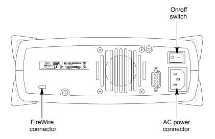
Figure 2-13 External FireWire drive: back-panel components
