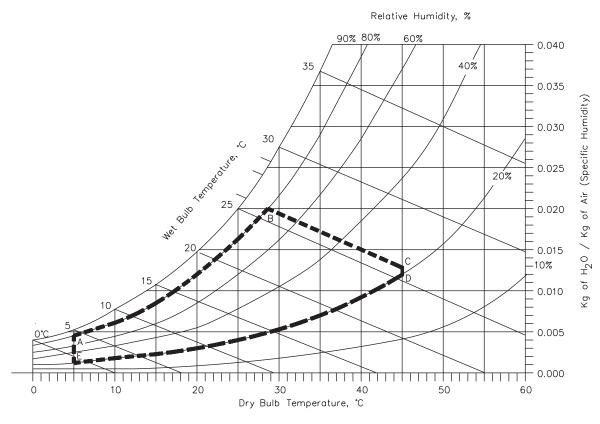
Figure 3-2 Temperature and humidity ranges for operation
