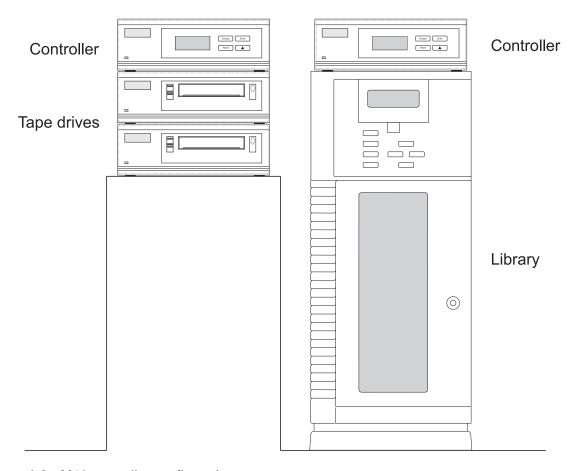
Figure 1-2 M10 controller configurations
