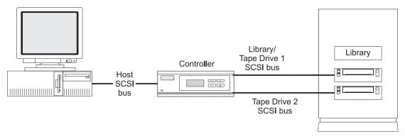
Figure 1-6 Actual configuration in pass thru mode
