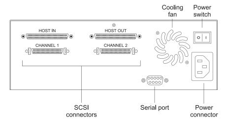
Figure 1-10 Back panel components
