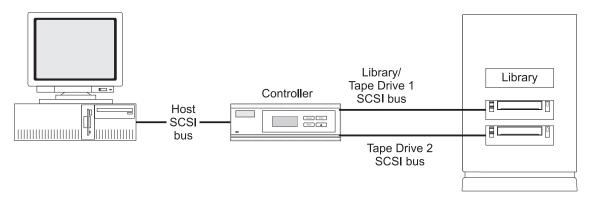
Figure 1-4 Actual configuration in mirroring mode
