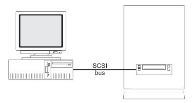
Figure 1-7 Configuration "seen" by the host in pass thru mode
