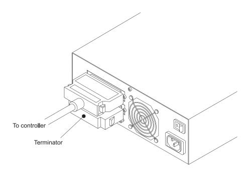
Figure 2-2 Tape drive connected to the controller
