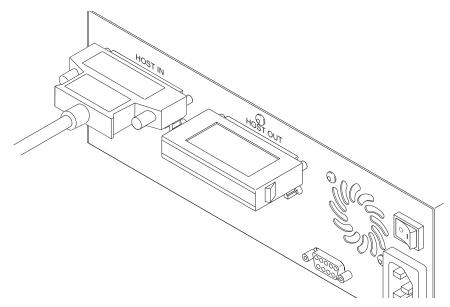
Figure 4-1 Termination of the host SCSI bus at the controller
