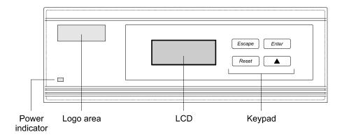
Figure 1-9 Front panel components
