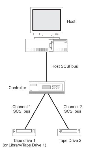
Figure 1-3 Controller position on the SCSI bus
