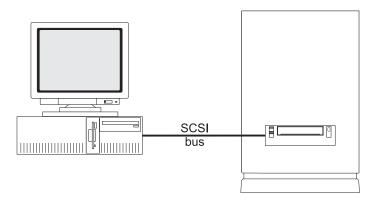
Figure 1-5 Configuration "seen" by the host in mirroring mode
