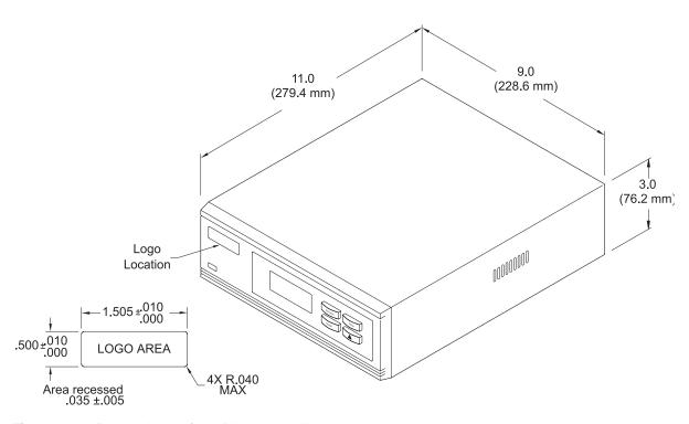
Figure 1-8 Dimensions of the M10 controller
