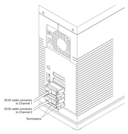
Figure 2-3 Library connected to the controller
