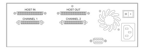
Figure 2-1 Controller SCSI connectors
