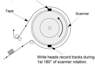
Exabyte's EXB-8200 helical scan recording provided read-after-write data verification
