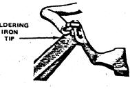
2. Apply only enough solder to thoroughly wet both the tip and the connection.
