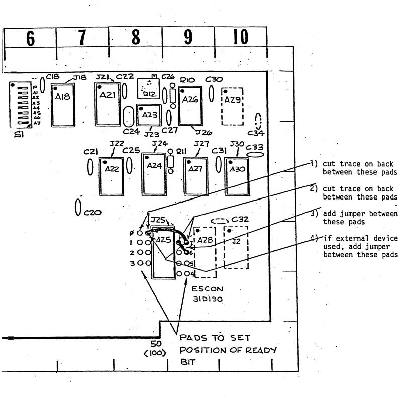
Figure 3. Changes Required to Adapt Interface Board to Correspond to the SIO port used in Altair Basic.
