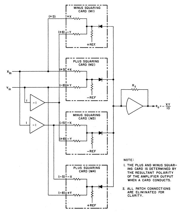
Figure 12. Four Quadrant Quarter-Square Multiplier, Simplified Schematic
