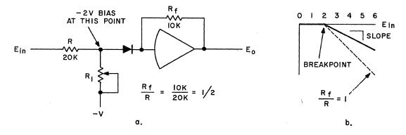
Figure 8. Simple Diode Function Generator
