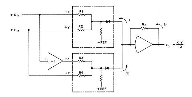
Figure 11. Two-Network Quarter-Square Multiplier, Simplified Schematic
