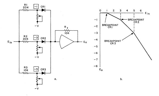
Figure 9. Three-Network Diode Function Generator
