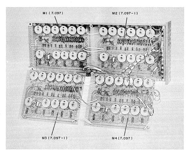
Figure 20. Multiplier With Card in Maintenance Position
