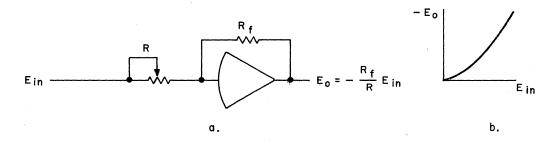
Figure 7. Elementary Function Generator
