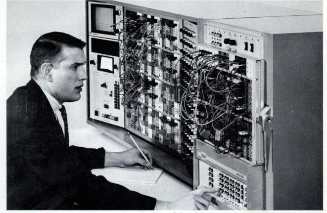
The DES-30 (Digital Expansion System) is a general-purpose, low-cost digital logic system. Though capable of operating autonomously, it was primarily designed as an expansion to the PACE<sup>®</sup> TR-48 Analog Computer - providing basic hybrid capabilities to the small computer facility. It is also readily combined with other generalpurpose analog or digital computers to provide extended control functions.
