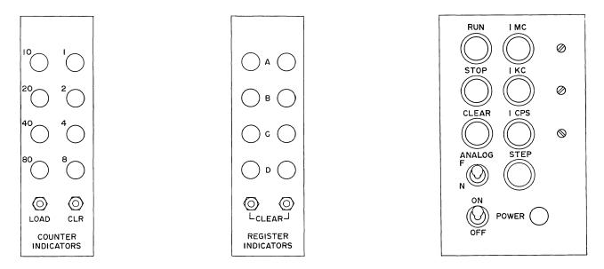
Figure 2. DES-30 Control Area (Field 3) provides control of timing, all clock frequencies, modes of operation and power. General purpose register and down counter indicators are also housed in this area.
