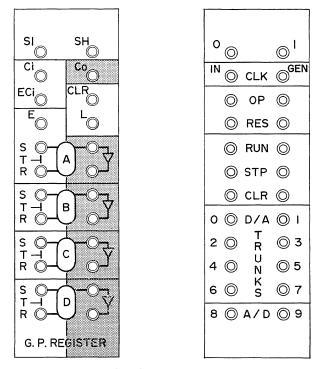
Figure 6. Field 2 Module Panel Layouts
