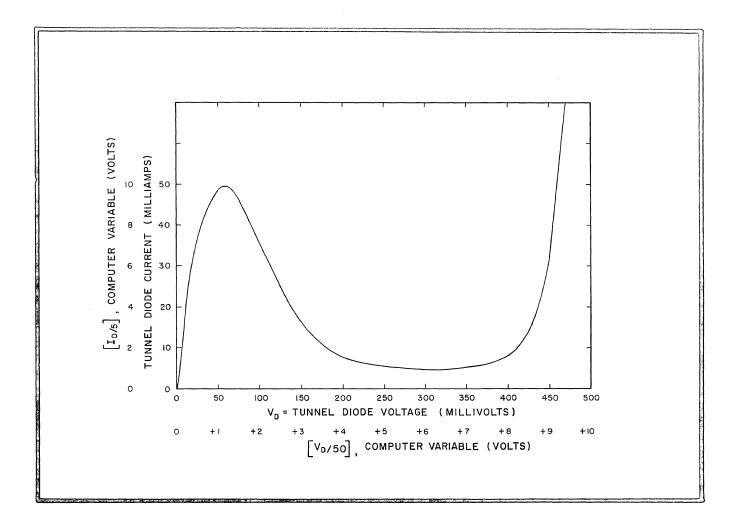
Tunnel Diode Curve Typifies Versatility of Variable Breakpoint Diode Function Generator
