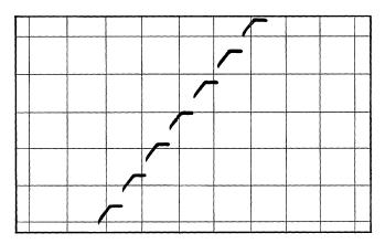
Output of 40.488 Used as Track. Hold Unit Sampling a Ramp at a 500 CPS Rate.
