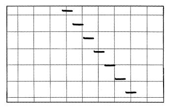
Output of Second Track-Hold Channel Which is Sampling Output of the First Track-Hold Channel (1) Controlled By Complementary Logic.
