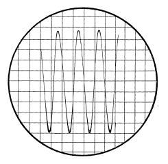
(Left) Output of 40.488 as Electronic Comparator Switching Between Same 1 KC Sinewave
