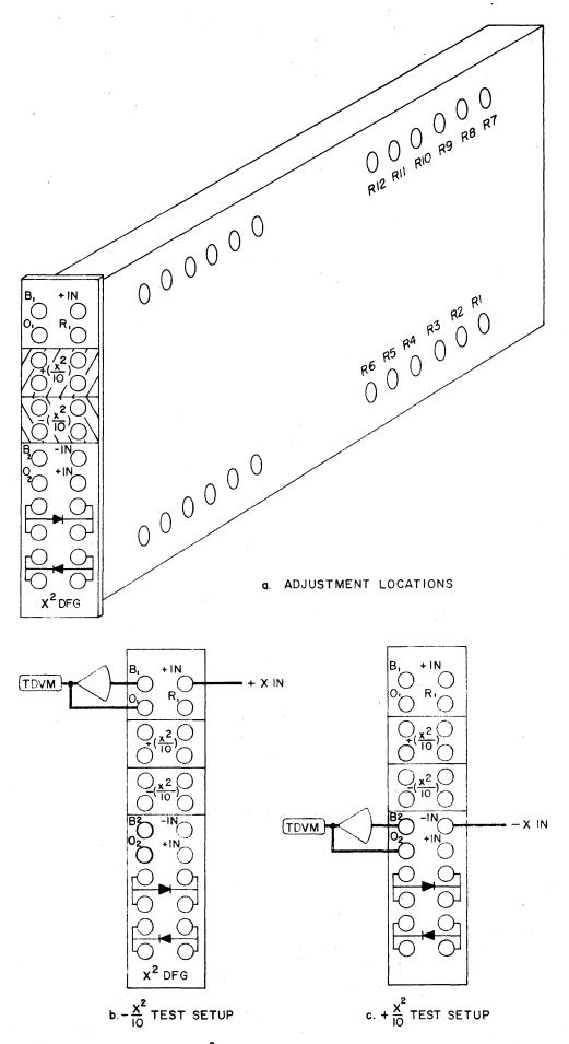
FIGURE 2.4-5 X<sup>2</sup> DFG ADJUSTMENT LOCATION AND PATCHING
