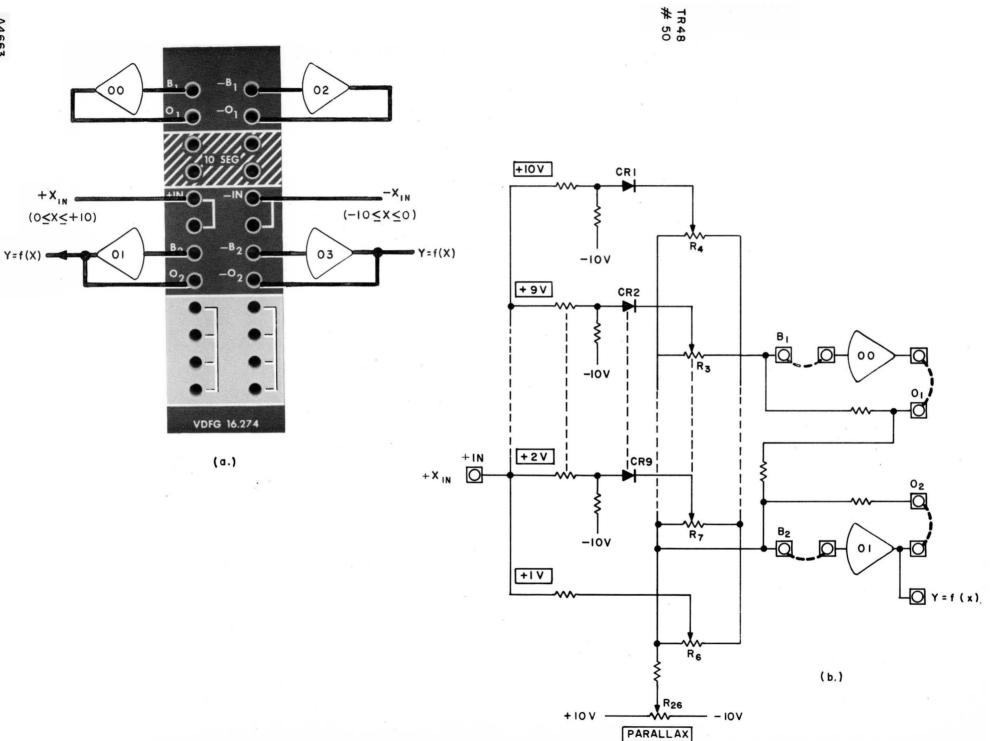
Figure 2.6-5 shows the VDFG patching to combine the plus and minus VDFG's for bipolar inputs. Note that a four-connector bottle plug covers the 10 SEG area of the patching block; one of the +IN terminations is jumpered to a -IN termination to combine the input leads.
