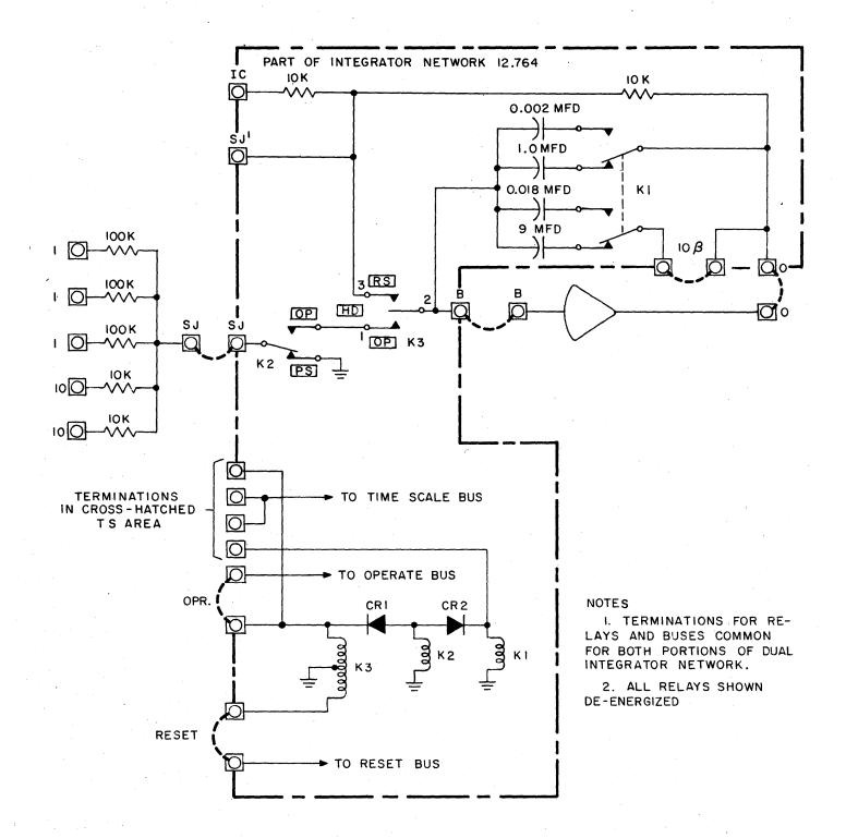
FIGURE 2. 2 - 2. INTEGRATOR, SIMPLIFIED SCHEMATIC
