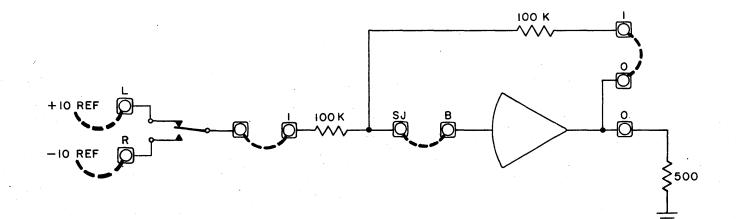
FIGURE 2.1-7 OUTPUT CURRENT TEST CIRCUIT
