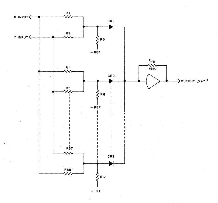
FIGURE 2.3-3. SIMPLIFIED PARTIAL-SCHEMATIC OF ONE SQUARING CIRCUIT
