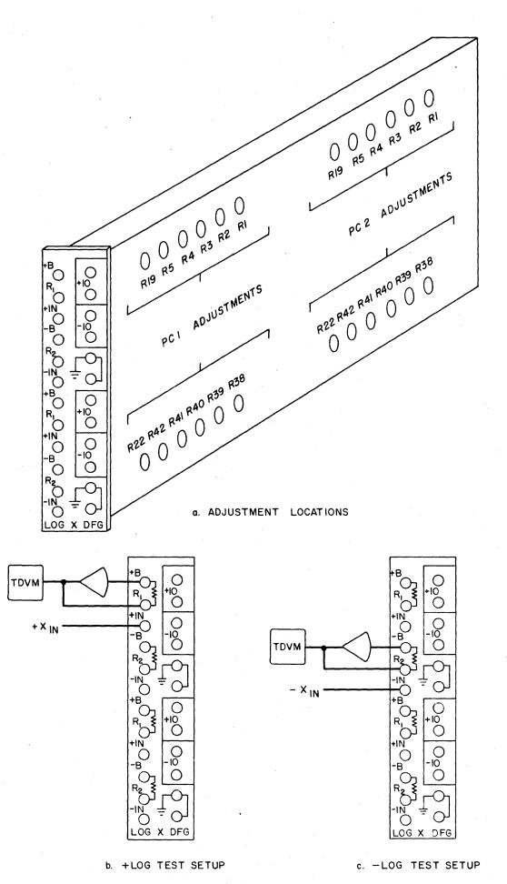
FIGURE 2.5-6 LOG X ADJUSTMENT LOCATION AND TEST SETUP PATCHING
