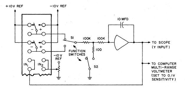
FIGURE 2.8-2 SIGNAL COMPARATOR TEST SETUP
