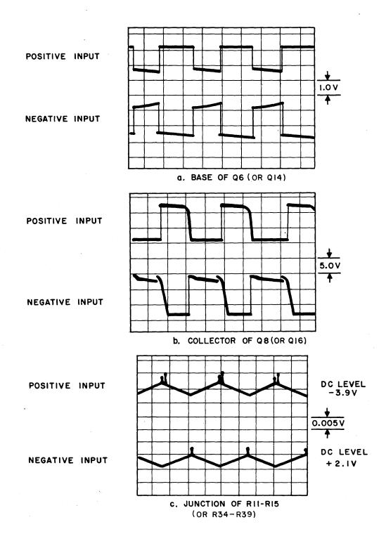
FIGURE 2.1 - 10 PROPERLY FUNCTIONING OVERLOADED STABLIZER WAVESHAPES
