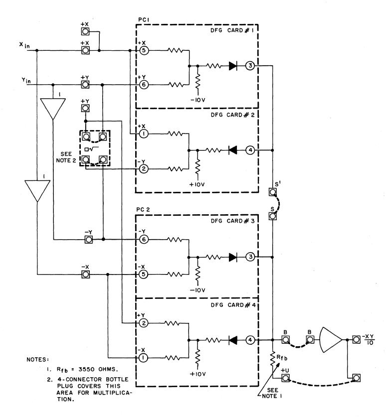
FIGURE 2.3-4. MULTIPLICATION PATCHING AND SIMPLIFIED SCHEMATIC.
