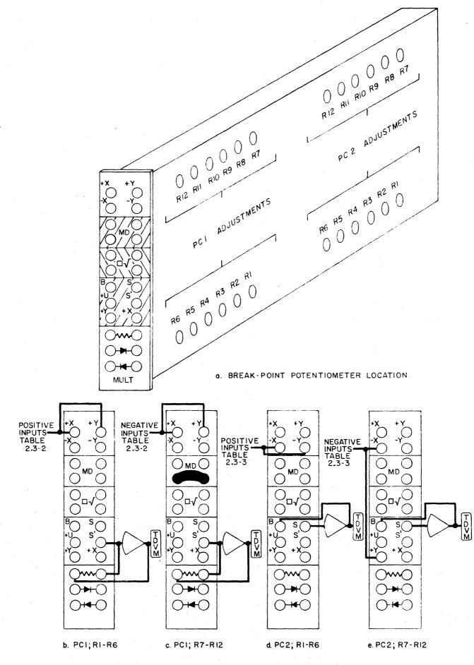
FIGURE 2.3-7 MULTIPLIER ADJUSTMENT LOCATION AND TEST SETUP PATCHING
