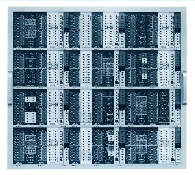
The removable patch panel is arranged as a series of 12 modules, with each module terminating a grouping of linear and non-linear computing components. This design coupled with logical component terminations assures maximum use of bottle plugs, thereby reducing patch panel clutter to a minimum even for large problems. Long, across-the-board patching is cut to a minimum. Problem patching, checking and trouble shooting are more easily accomplished and there is less chance of patching error.
