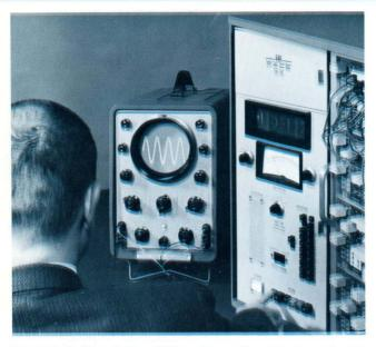
The High Speed Repetitive Operation Group permits the PACE TR-48 to be operated alternately as a realtime or high speed repetitive computing device. The wide bandwidth of the TR-48 solid-state computing components is utilized to produce problem solutions many times each second . . . yet there is no loss in time computing accuracy.
