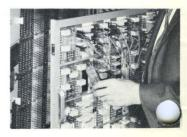
Snap out the patching block of the component to be replaced and replace it with a block for the desired component.
