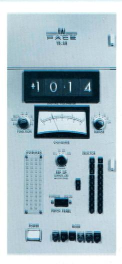
**Control Panel** is the nerve center of the TR-48 Computer . . . placing all controls for the complete operation of the computer in one convenient location. Human engineered panel design facilitates computer utilization and problem solution . . . provides means for controlling computer operation and metering of component output voltages. All knobs, push-buttons, and switches are clearly labeled for easy identification.
