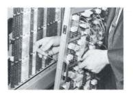
Loosen the pre-patch panel retaining frame.
