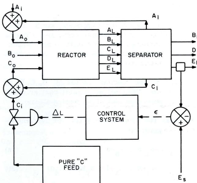
Figure 1: Block Diagram of Physical System
