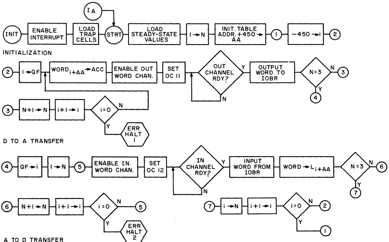
Figure 8: Flow Diagram of Digital Program
