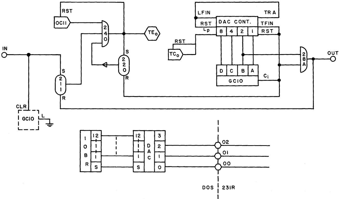
Figure 6: DAC Circuit
