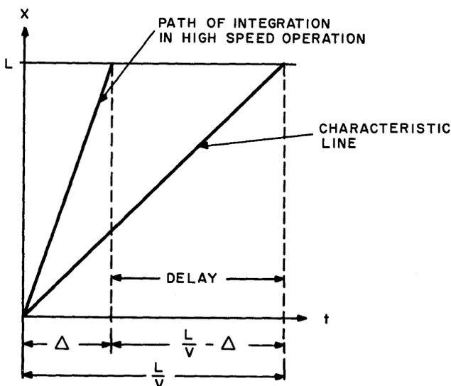
Figure 4: Diagram of High-Speed Computing Technique
