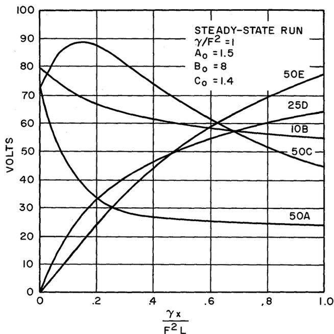
Figure 9: Steady-State Concentrations Versus Reactor Length Variable
