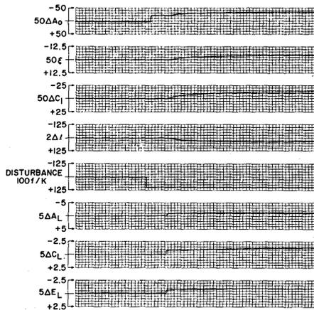
Figure 12: Run 4, System Response to Step Input ( $K_c = 10$ )
