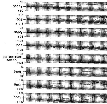
Figure 14: Run 6, System Behavior with Improper Control Settings
