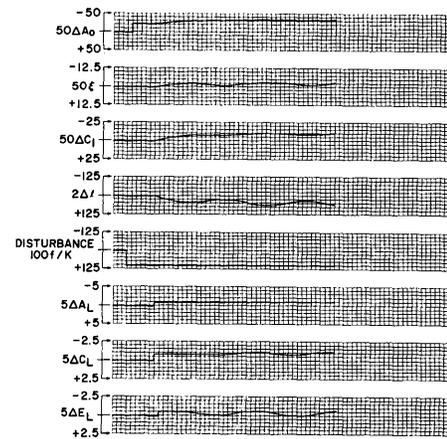
Figure 13: Run 5, System Response to Step Input ( $K_c = 20$ )
