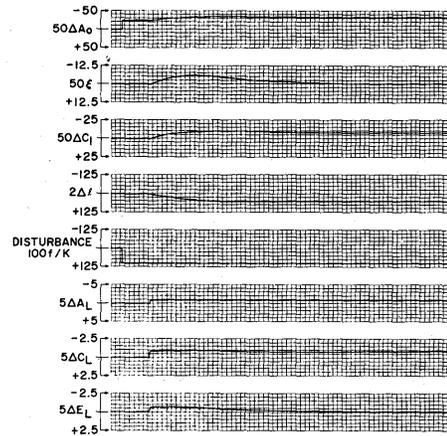
Figure 15: Run 7, System Response to Step Input ( $K_c = 10, T_r = 5$ )
