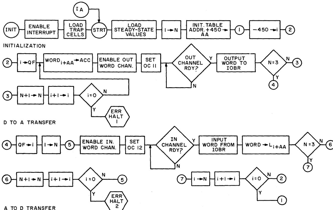
Figure 8: Flow Diagram of Digital Program
