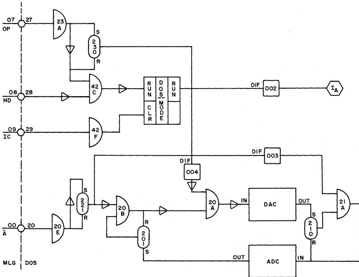
Figure 7: Conversion Timing and Initialization Circuit
