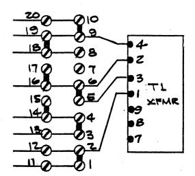
WIRING CONFIGURATION 230 VAC 50-60 HZ
