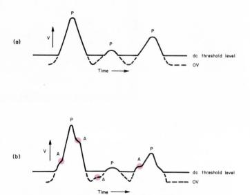
Fig. 1. The upper waveform, (a), is a good NRZI playback signal, after rectification. Note that zero-slope points, P, occur only at the true peak of the waveform. Waveform (b), on the other hand, shows spurious zero-slope points, A, from vibration, crosstalk, and dropouts. These cause unwanted outputs from conventional peak detectors.
