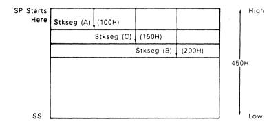
Figure 7-3. Combining Segments with Stack Combination
