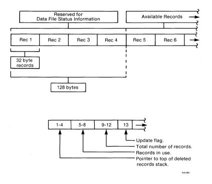
Figure 3-2. Sample Data File Layout for 32-byte Records
