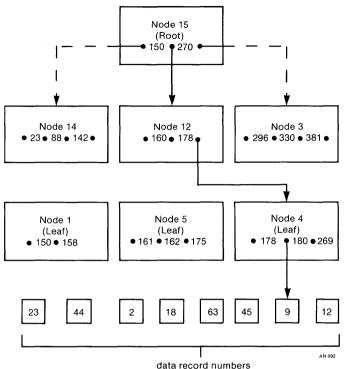
Figure 1-1. B+ Tree Structural Diagram
