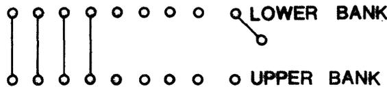
9.  Use the leads clipped from the bypass capacitors in Step 6, or wire of approximately 28 - 30 gauge, to connect the jumpers according to the scheme as presented above. Solder the jumpers and clip off the excess leads.
