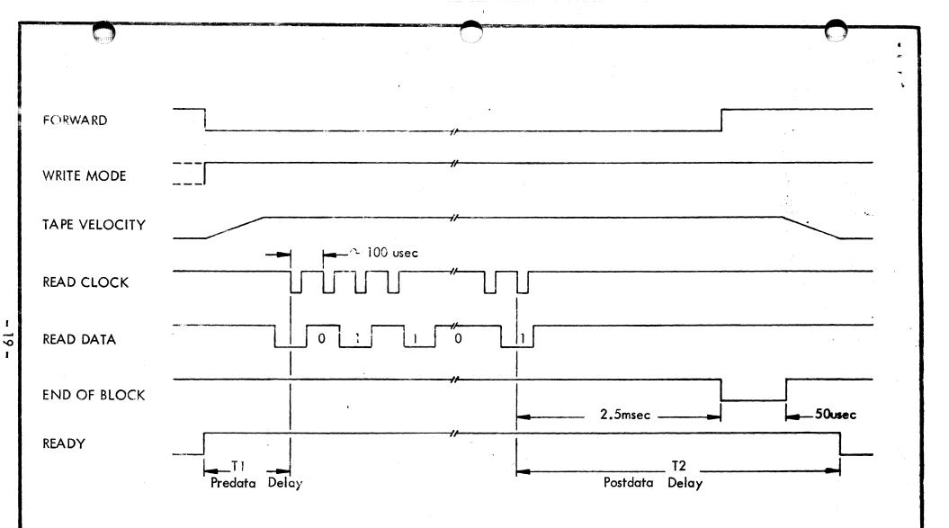
Figure 3. Read Operation Timing Diagram
