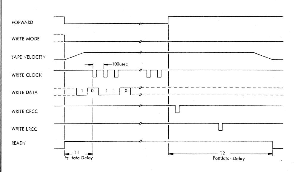
Figure 2. Write Operation Timing Diagram
