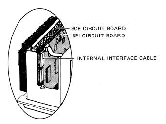
Figure 1-3. Model 630 SPI CIRCUIT BOARD LOCATIONS
