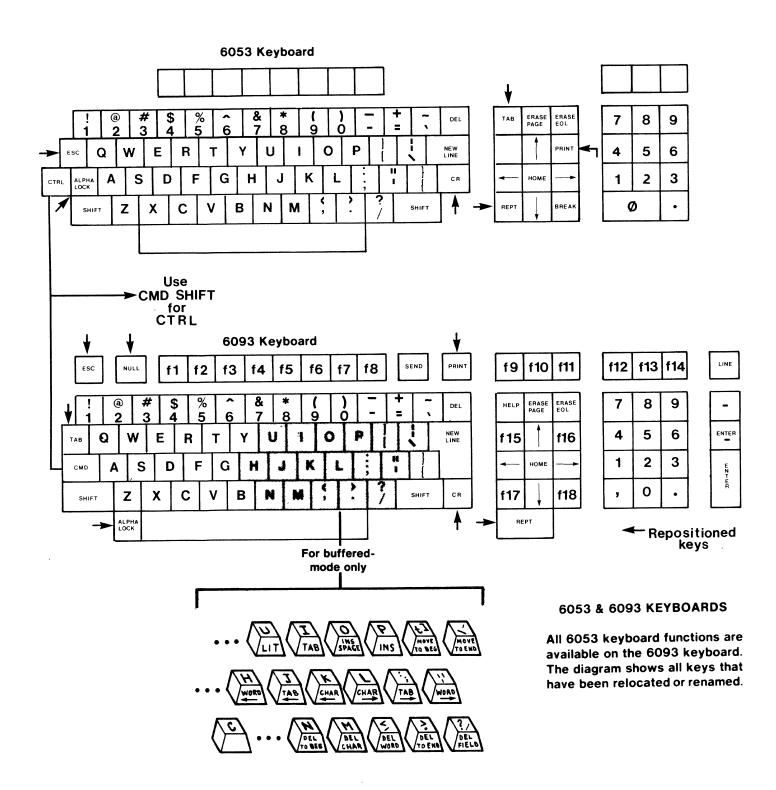
Figure 1 Dasher D3 (6093) Display Terminal Keyboard
