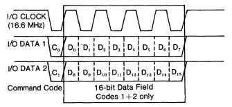
The IOCs provide full decoding of this command stream, making bus protocol transparent to the user. The IOC provides a fully parallel 16-bit data bus for device interfacing and incorporates common controller functions for programmed I/O, program interrupt, and data channel (DMA) functions.
