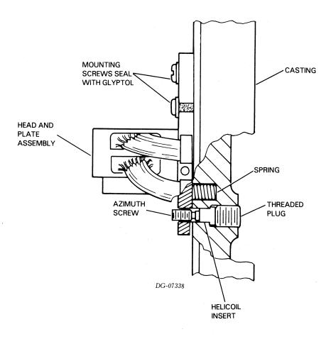
4. Remove the three screws holding the head and its mounting plate to the casting. Carefully lift the head away from the casting and recover the spring from behind the head plate. Slip the head cables through the opening in the casting.
