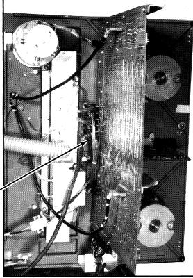
6. Adjust the column position trimpots (R65 R673), so that the two loops line up with the center bolts on the liners.
