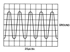
5. Adjust trimpot R651 so that the amplitude of the wave form is 10.0 volts, peak to peak.
