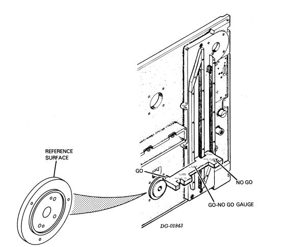
11a. Place the take up reel and the hub cover plate on the hub and tighten the mounting screws to 10 in-lbs.
