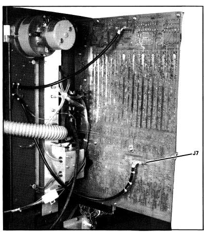
Connect Channel 1 of the scope to the data reading path test point for channel 4 (TP-14). Connect Channel 2 of the scope to channel 5 (TP-15).
