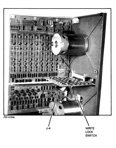
3. Put the new switch in place and replace the two retaining screws.
