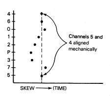
Possible skew pattern after aligning outside channels.
