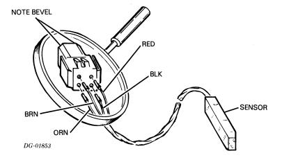
3. While holding the sensor unit, remove its retaining screw and pass its wires through the casting one at a time.
