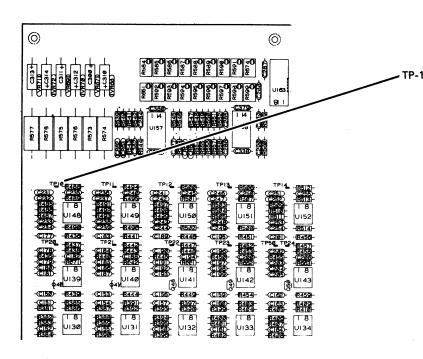
3. Swing open the casting and place a probe on TP-10. Use the command string (see Appendix C) to write all 1's on tape and verify that the signal is present in the data ground reading circuit.
