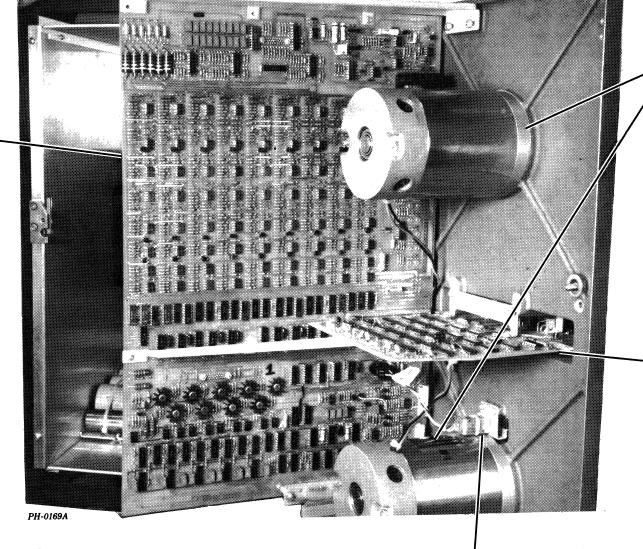
WRITE LOCK SWITCH Enables the write circuitry when write ring is installed on supply reel.
