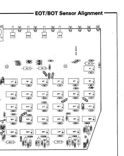
6. Use the digital multimeter to observe the voltage levels of TP-1 and TP-2 on the console board. If they are not within 5%, loosen the sensor retaining screw and adjust the sensor to get the two signals as equal as possible. Tighten the retaining screw and recheck the voltages.
