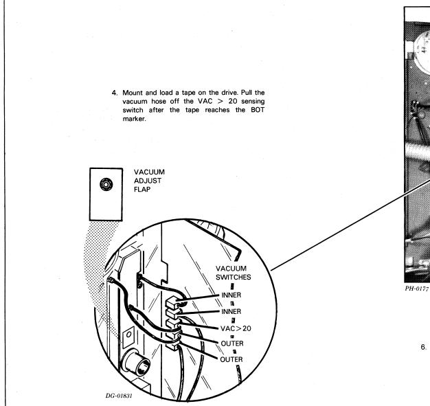
5. Connect the vacuum hose to the vacuum gauge. Loosen the vacuum flap retaining nut and adjust the vacuum flap for a reading of 30 inches on the gauge. Tighten the nut and reconnect the hose to the vacuum switch.
