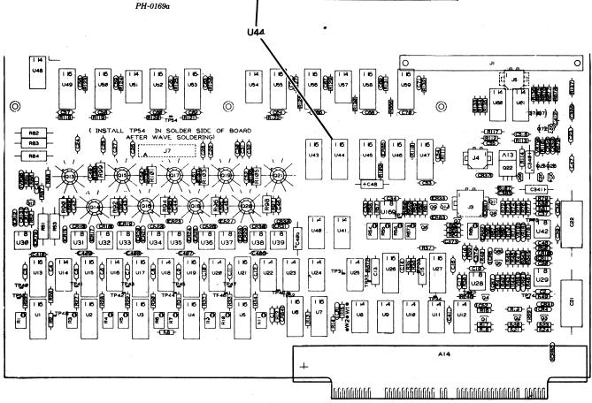
12.Connect Channel 1 of the scope to U44 pin 9.
