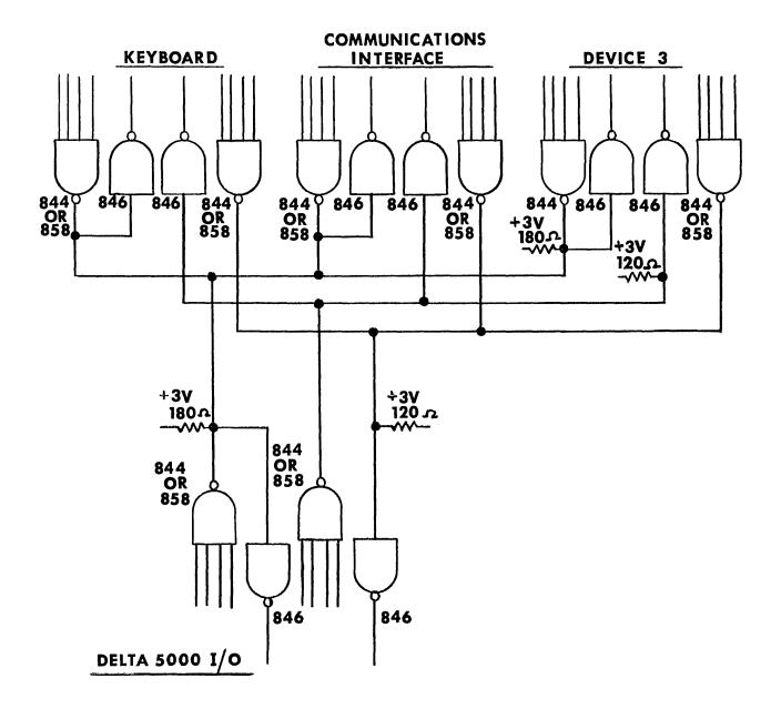
FIGURE 8-1 PARTY LINE LOADING INTERCONNECTING DIAGRAM
