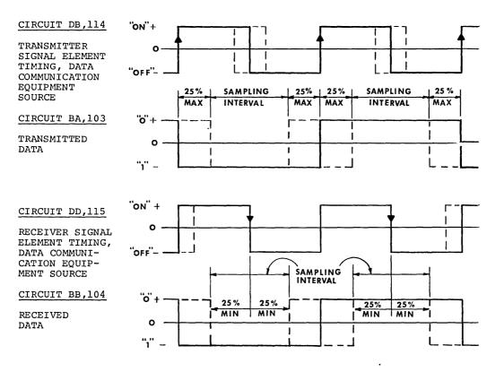
FIGURE 7-2. COMMUNICATIONS TIMING DIAGRAM
