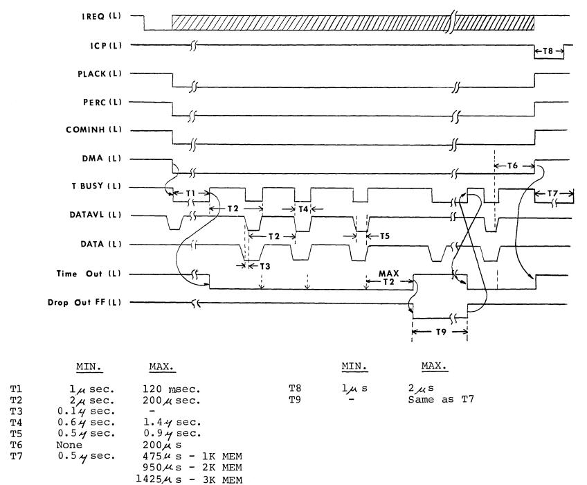
FIGURE 8-5 DMA RECEIVE TIMING DIAGRAM
