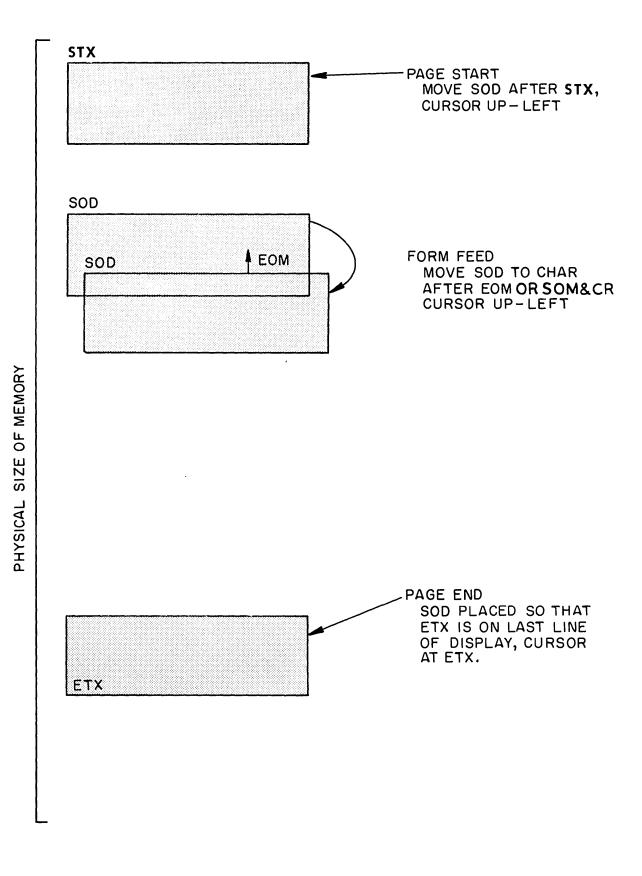
Figure 4-2 Example of Display Window
