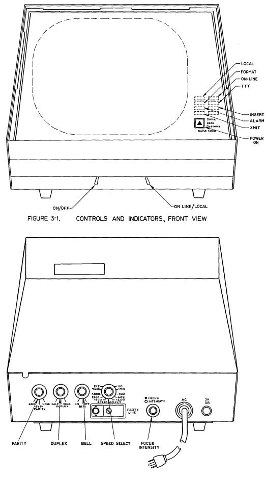
FIGURE 3-2. CONTROLS, REAR VIEW
