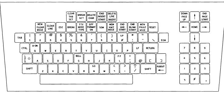
of the typewriter numeric keys. Above the number pad are the cursor and paging control keys.
