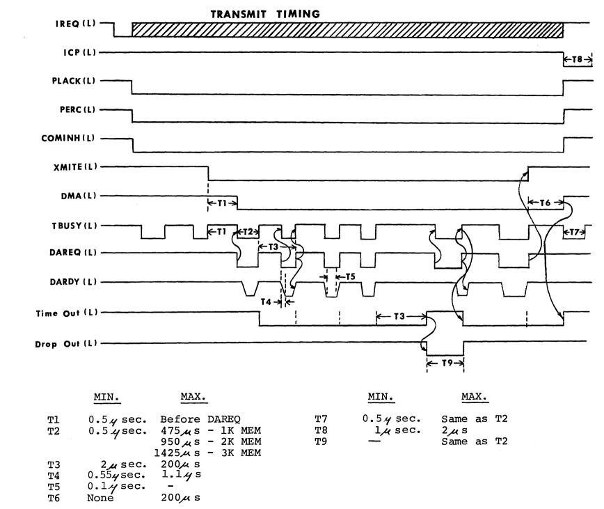
FIGURE 8-6 DMA TRANSMIT TIMING DIAGRAM
