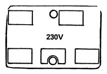
PC card position for line voltage 210 - 260 Volts. Use 1 A slo blo fuse.
