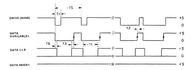
FIGURE 4-2 PULSE DRIVE TIMING DIAGRAM
