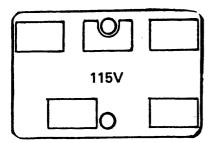
PC card position for line voltage 105 - 130 Volts. Use 2 A slo blo fuse.
