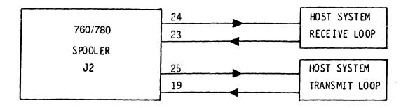
For passive operation (current supplied by host system), S3-7 and S3-8 are open.
