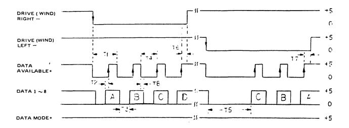
FIGURE 4-1 SPOOL MODE TIMING DIAGRAM (LEVEL OPERATION)
