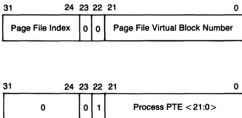
Figure 14-10 Possible Contents of PFN BAK Array Element
