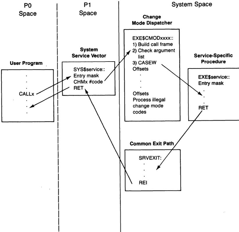
Figure 9-1 Control Flow of System Services That Change Mode
