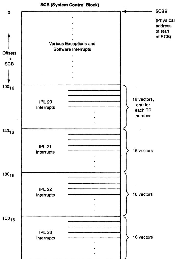
A second SCB page exists on the VAX-11/730 and VAX-11/750 for directly vectored UNIBUS device interrupts. A VAX-11/750 with a second UNIBUS will have a third SCB page for interrupts on the second UNIBUS.
