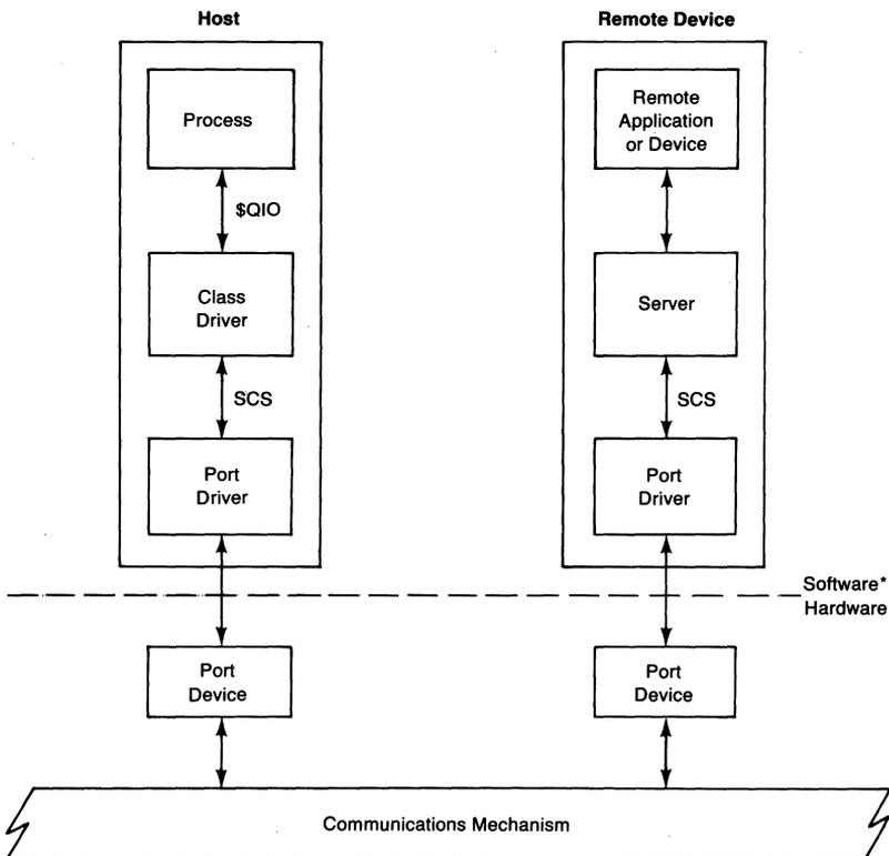
\*It is possible for the remote device to implement the port driver and server in hardware.
