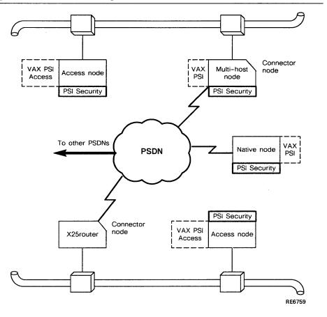
Figure 4–1 VAX PSI Configurations and Access to PSDNs
