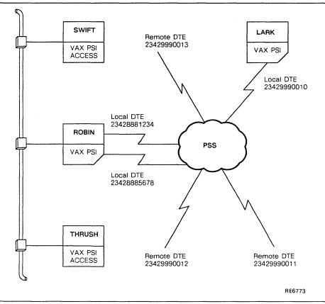
Figure 6–1 An Example of a Typical PSI Installation
