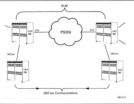
The DECnet Routing module recognizes that the data has to go through a PSDN and selects a DLM circuit to carry the data. The DLM circuit passes the DECnet data to the VAX PSI software for conversion to X.25 packets. This is done by including X.25 protocol information with the DECnet data. VAX PSI then sends the packets to the remote DTE, which removes the X.25 protocol information before sending the DECnet data on to its destination.
