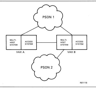
Combination nodes provide additional flexibility as they operate either as Connector or Access nodes:
