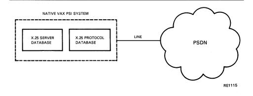
After a Native mode system has been installed you need to add destinations to the X25-SERVER database. Destinations are used to receive incoming calls to the VAX PSI software from remote DTEs. If a call matches a destination, then a process associated with the destination is activated.
