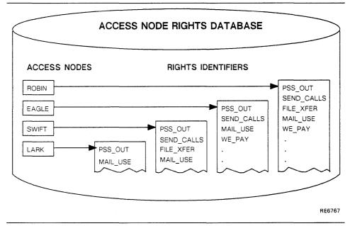
In Figure 5–5, the Access nodes are ROBIN, EAGLE, LARK and so on. Each Access node has a list of rights identifiers such as PSS\_OUT, SEND\_CALLS, FILE\_XFER and so on. The access actions associated with these rights identifiers are specified in the ACLs contained in the Object Access Control Databases.
