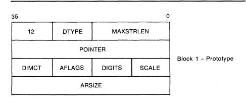
Figure 2–12 Varying String Array Descriptor Format
