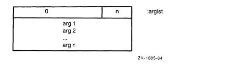
The first longword is always present and contains the argument count as an unsigned integer in the low byte. The 24 high-order bits are reserved to DIGITAL and must be zero. To access the argument count, the called procedure must ignore the reserved bits and access the count as an unsigned byte (for example, MOVZBL, TSTB, or CMPB). The remaining longwords can be one of the following:
