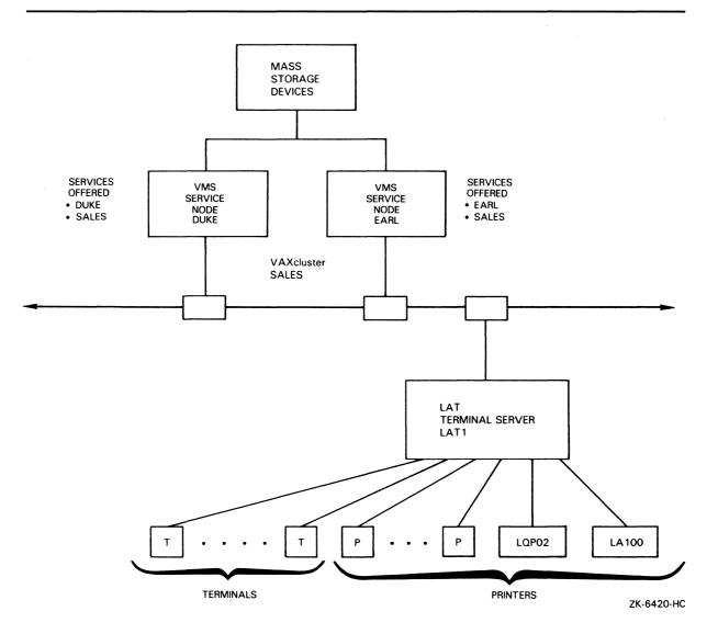
Figure 2–1 Service Nodes, Remote Printers, and Services
