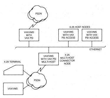
Figure 6-11 • DECnet Network Configuration Showing Examples of X.25 Connections
