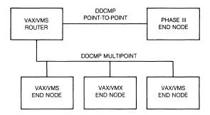
Figure 6-9 • Typical DDCMP Point-To-Point Connections
