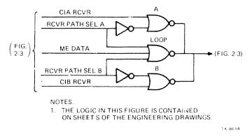
Figure 2-4 Receive Path Select Mux-ECL Logic
