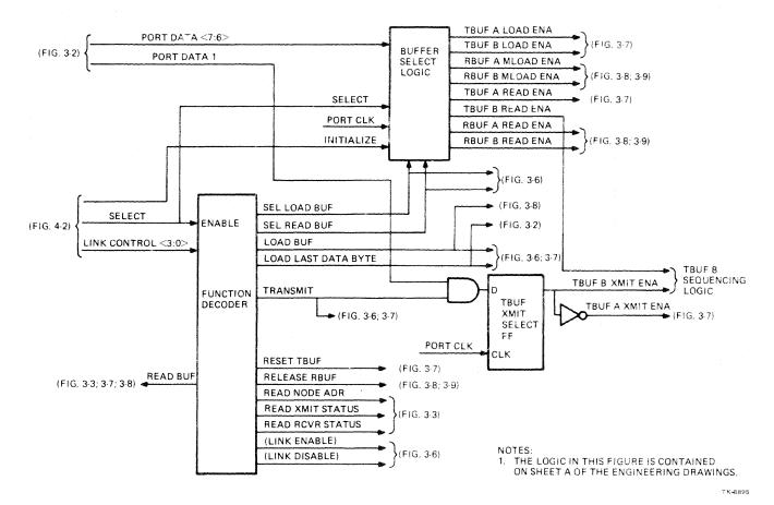
Figure 3-5 Function Decoder and Buffer Select Logic
