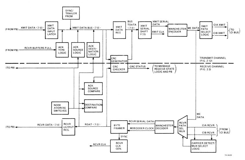
Figure 2-2 Link Simplified Block Diagram
