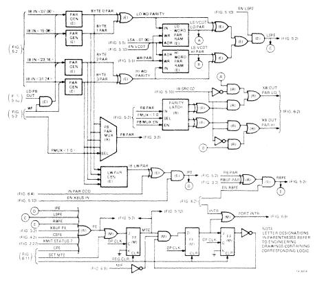
Figure 5-11 Parity Generator/Checker Logic
