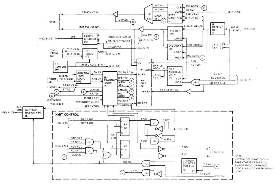
Figure 6-2 Write Transfer Block Diagram
