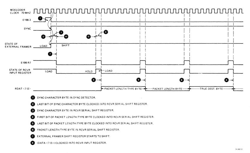
Figure 2-9 Byte Framer Timing Diagram
