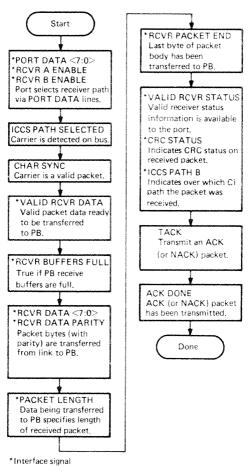
Figure 2-24 Interface Flow Diagram - Receive Operation
