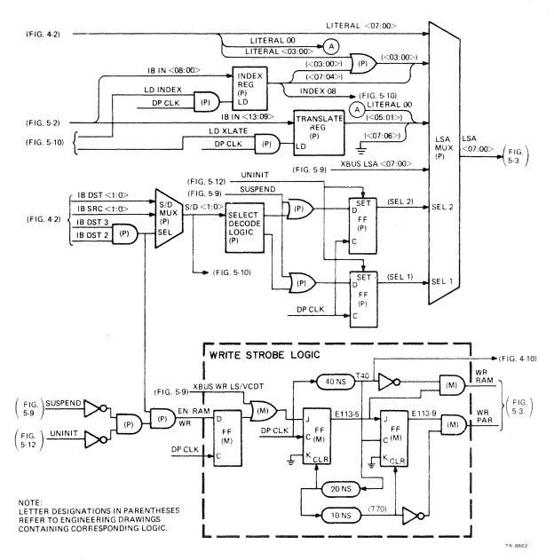
Figure 5-5 LS/VCDT Address Selection Block Diagram
