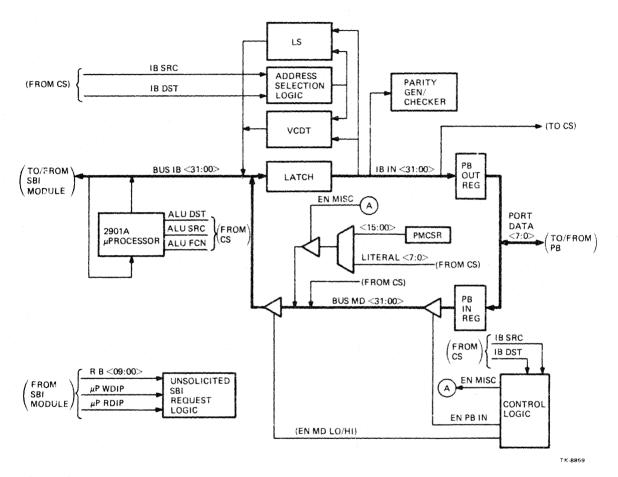
Figure 5-1 Data Path Block Diagram
