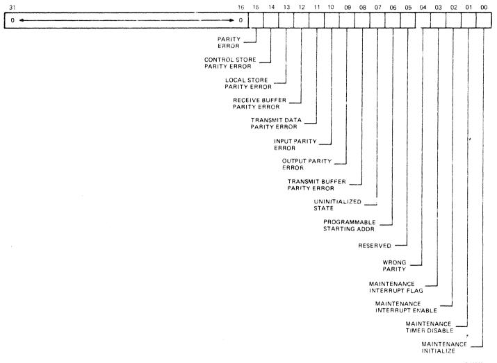
Figure C-3 Port Maintenance Control/Status Register (PMCSR) Bit Fields TK-9912
