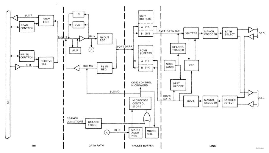
Figure 1-4 CI780 Block Diagram
