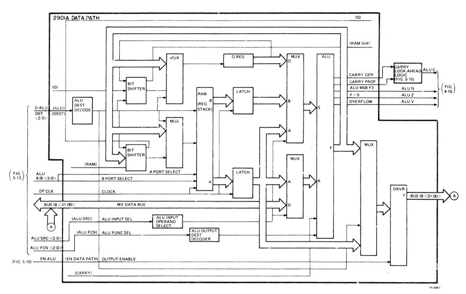
Figure 5-14 2901A Microprocessor Block Diagram
