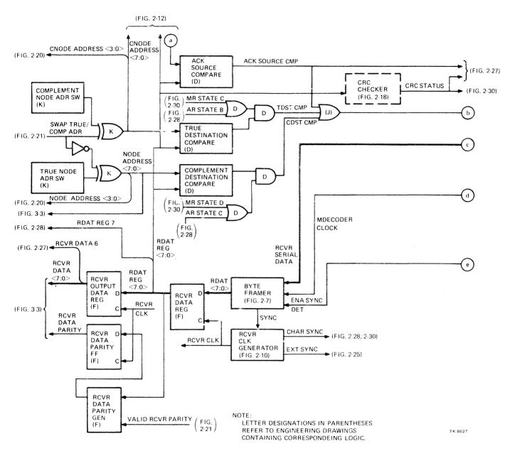
Figure 2-3 Receive Channel Block Diagram (a)
