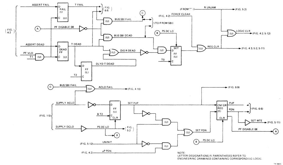
Figure 6-11 Initialization and Restart Logic
