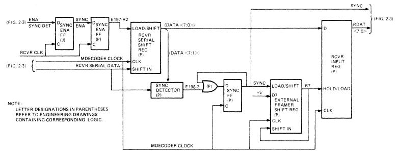
Figure 2-7 Byte Framer Block Diagram
