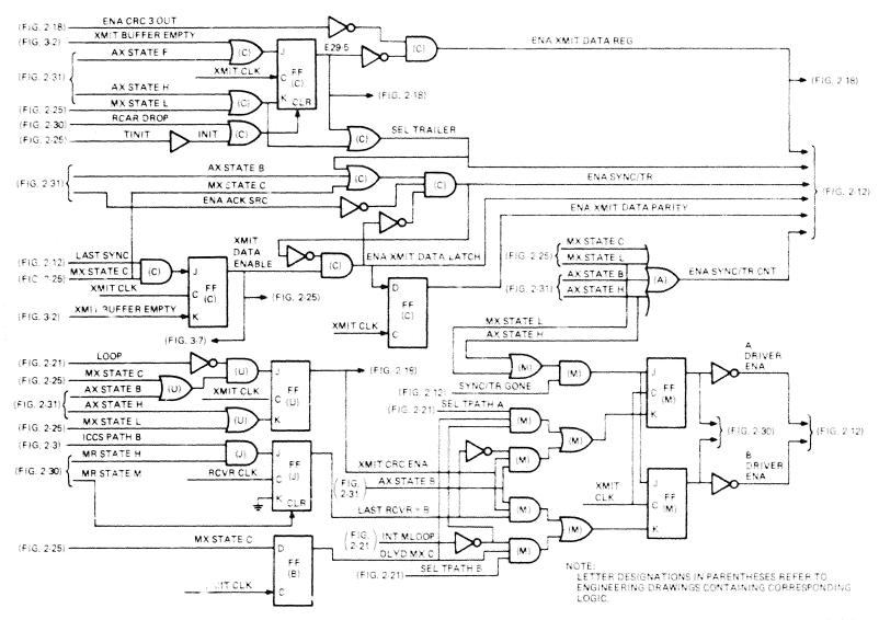
Figure 2-26 Transmit Control Logic
