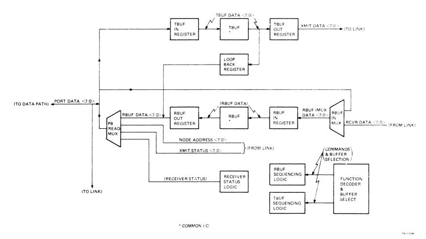
Figure 3-1 Packet Buffer Data Flow
