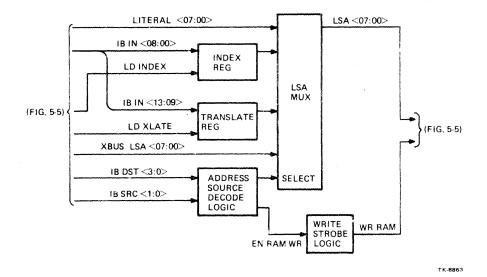
Figure 5-4 LS/VCDT Address Selection Simplified Block Diagram
