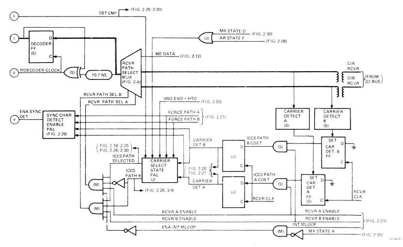
Figure 2-3 Receive Channel Block Diagram (b)
