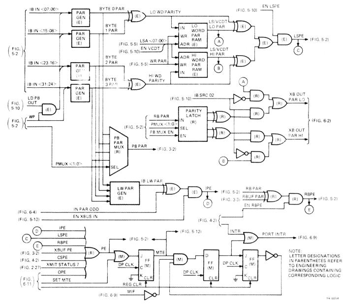
Figure 5-11 Parity Generator/Checker Logic
