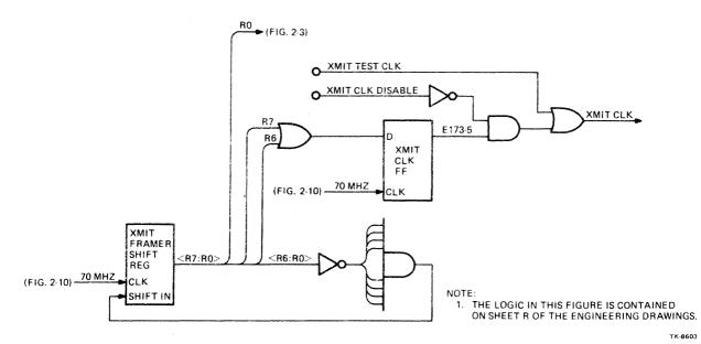
Figure 2-14 XMIT CLK Generator Block Diagram
