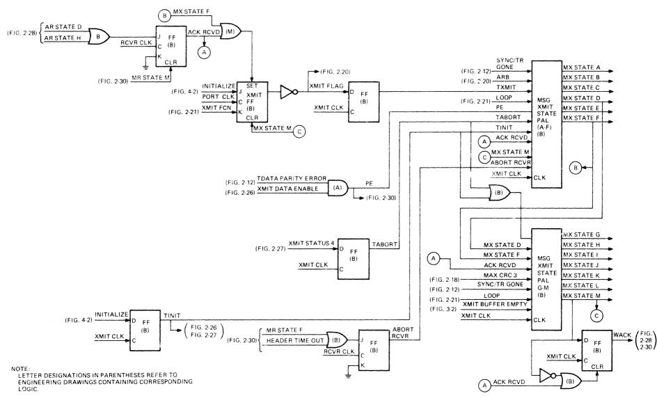
Figure 2-25 Message Transmit State Logic
