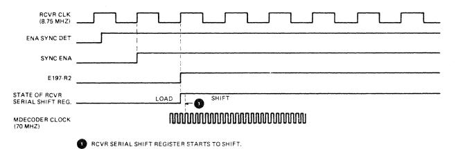
Figure 2-8 Enabling the RCVR Serial Shift Register
