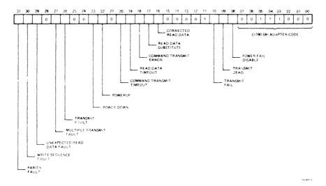
Figure C-4 Configuration Register (CNFGR) Bit Fields
