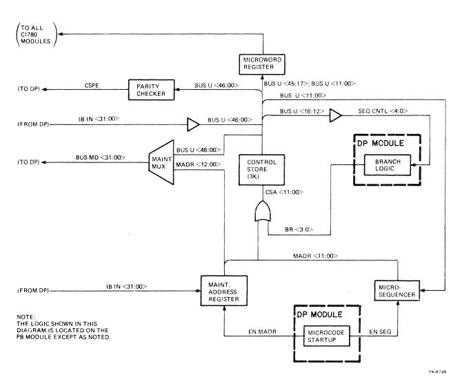
Figure 4-1 Control Store Simplified Block Diagram
