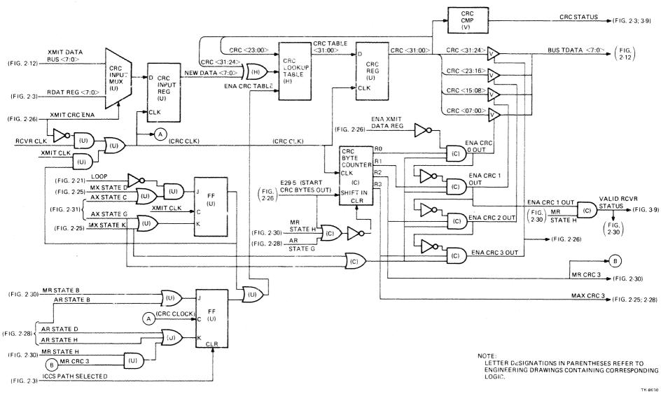
Figure 2-18 CRC Generator/Checker
