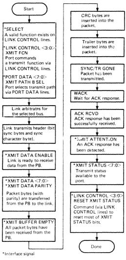
Figure 2-23 Interface Flow Diagram - Transmit Operation
