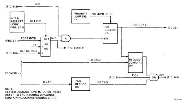
Figure 6-9 ISR Block Diagram
