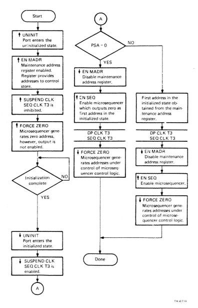
Figure 4-11 Microcode Start-Up Fiow Diagram
