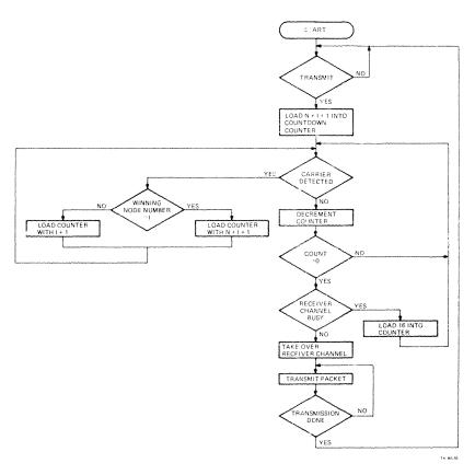
Figure 2-19 Arbitration Flow Diagram
