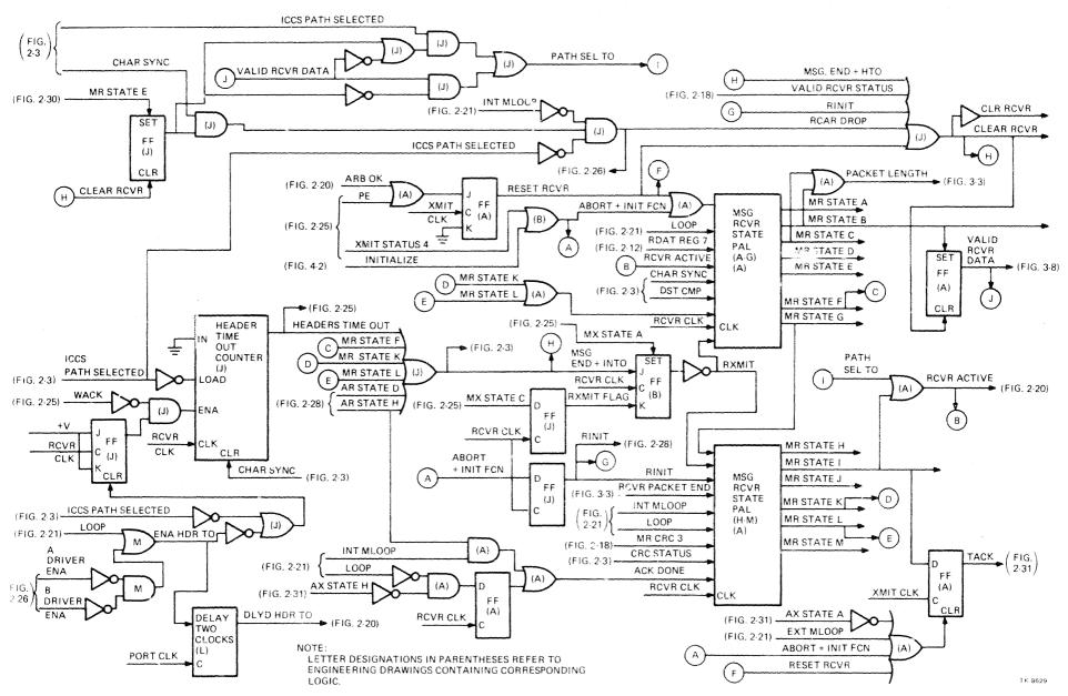
Figure 2-30 Message Receive State Logic
