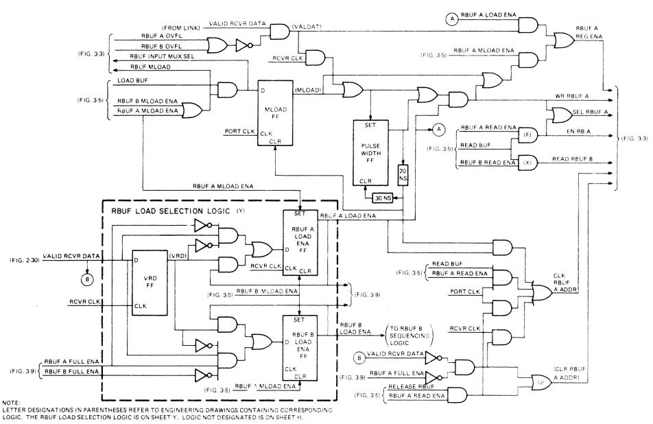
Figure 3-8 RBUF Sequencing Logic
