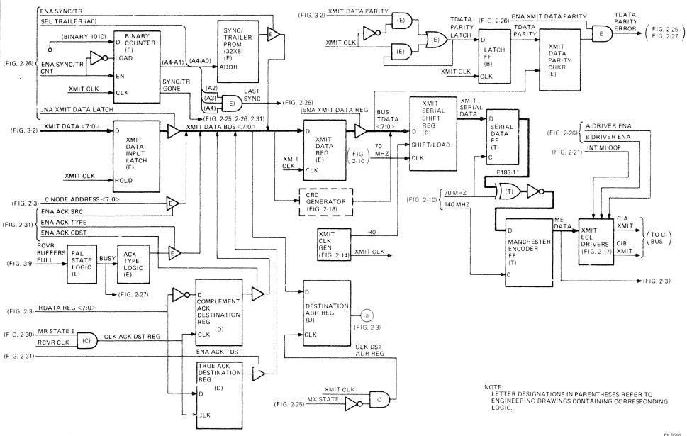
Figure 2-12 Transmit Channel Block Diagram
