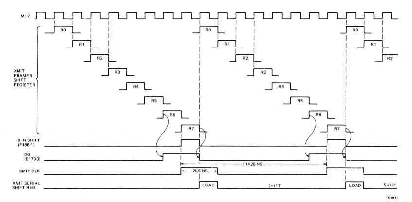
Figure 2-15 XMIT CLK Generator Timing Diagram
