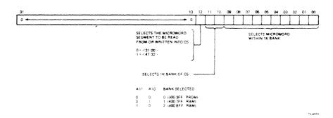
Figure C-1 Maintenance Address Register (MADR) Bit Fields
