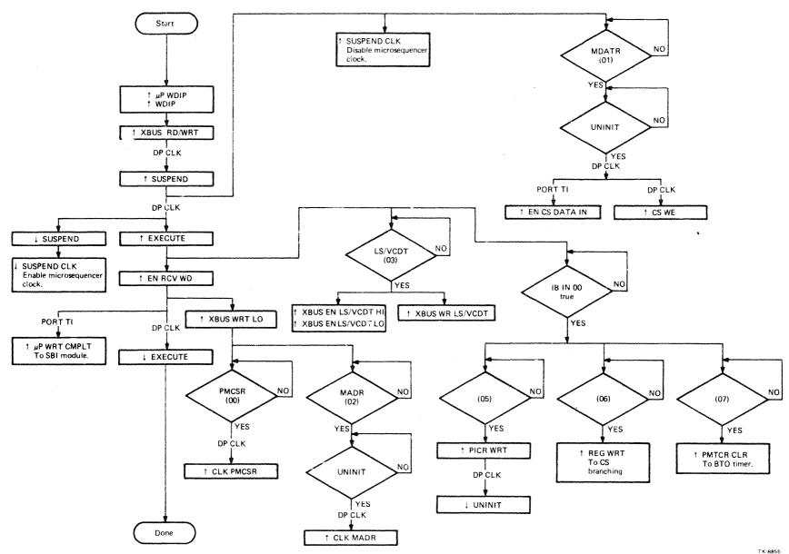
Figure 5-7 Unsolicited SBI Write Request Flow Diagram
