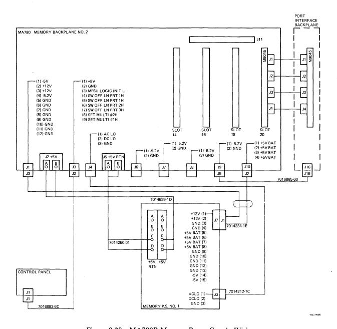
Figure 9-28 MA780B Memory Power Supply Wiring
