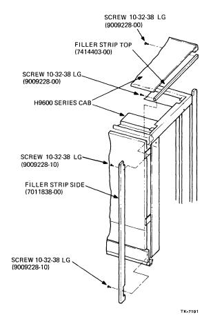
Figure 9-5 H9504-XE Filler Strip Installation
