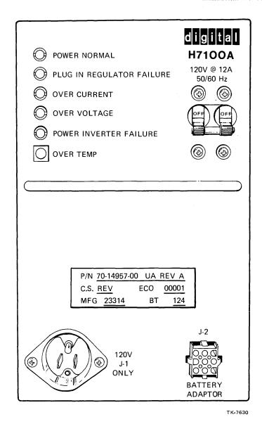
Figure 9-29 Memory Power Supply (Front View)
