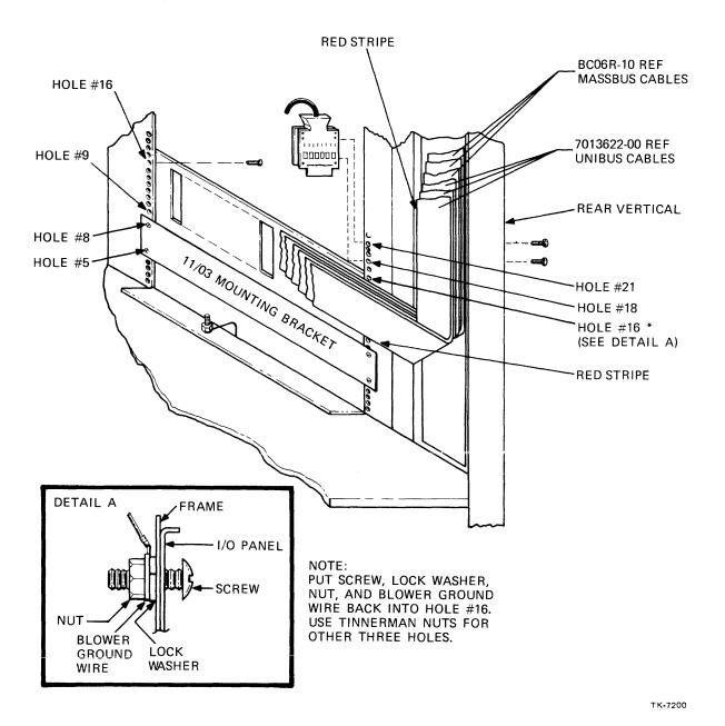
Figure 9-36 Left I/O Panel Installation
