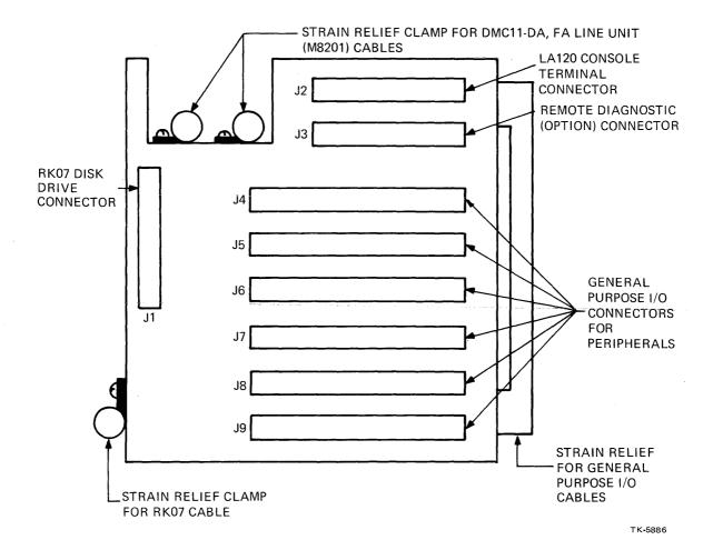
Figure 10-4 I/O Panel Assembly Connectors
