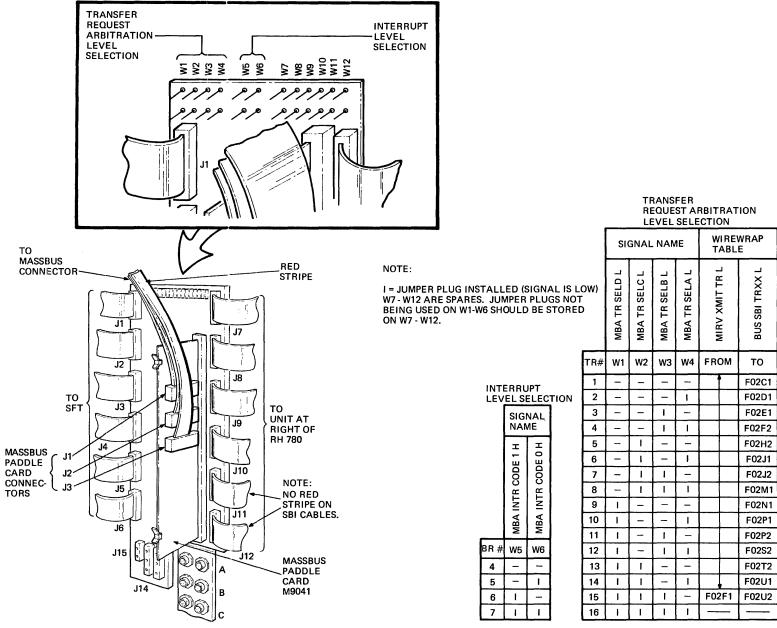
Figure 7-2 Transfer Request Arbitration, Interrupt Level Details
