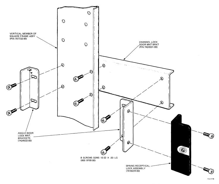
Figure 9-10 H9504-XE Door Locking Bracket Installation
