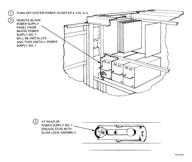
Figure 4-2 FP780 Installation (Sheet 1 of 4)
