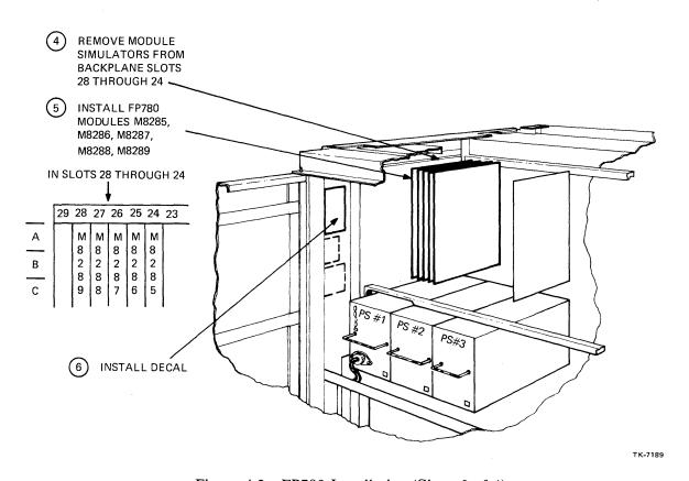
Figure 4-2 FP780 Installation (Sheet 2 of 4)
