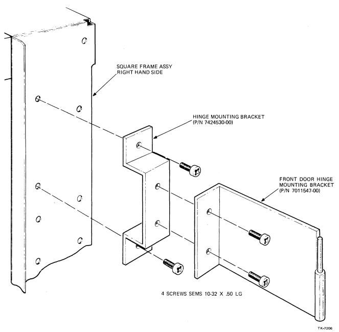
Figure 9-12 H9504-XE Front Door Hinge Installation
