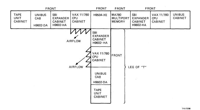
Figure 9-4 Three VAX-11/780 "T" Arrangement
