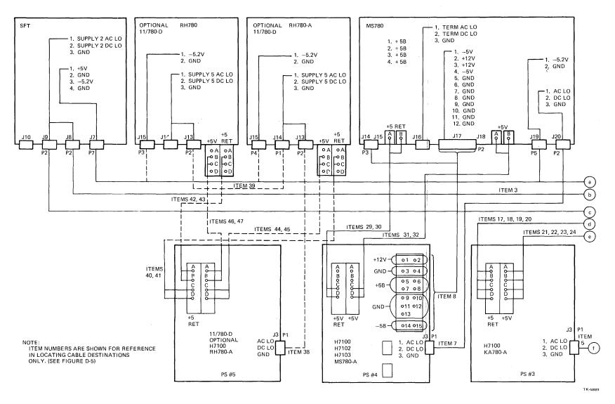
Figure 12-3 VAX-11/780 Subsystem Backplane DC Interconnect Diagram (Sheet 1 of 2)
