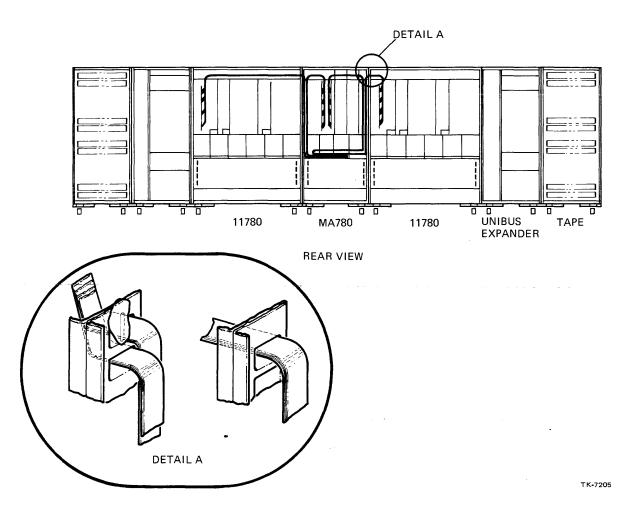
Figure 9-2 Two-System BDI Cable Routing
