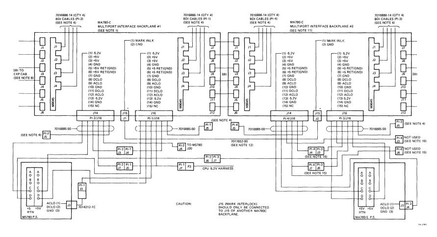
Figure 9-34 MA780C Power Cables with Four Ports on SBI
