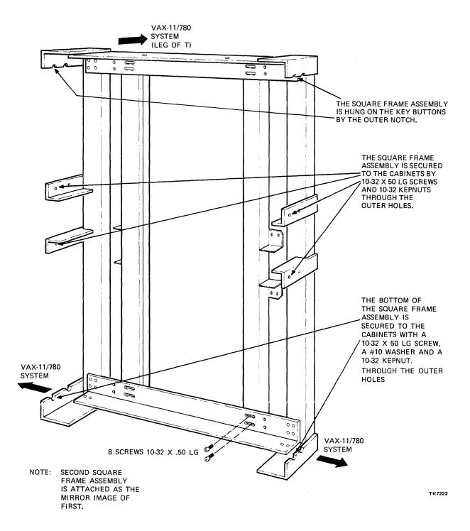
Figure 9-8 H9504-XE Square Frame Assembly Installation
