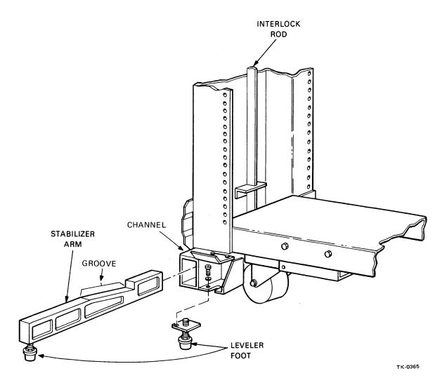
Figure 1-6 Stabilizer Arm and Leveling Pad
