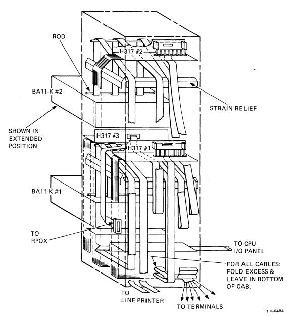
Figure 1-8 UNIBUS Expander Cabinet Cabling
