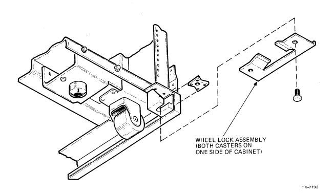
Figure 1-3 Wheel Lock Assembly
