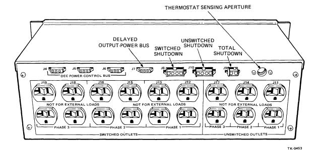
Figure 9-31 869D Power Controller (Front and Back Views)
