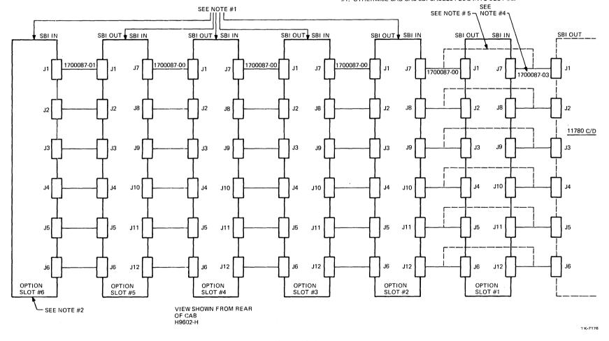
Figure 5-7 Ribbon Cable Interconnections
