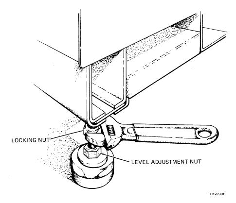
Figure 1-2 Leveling Feet Adjustment
