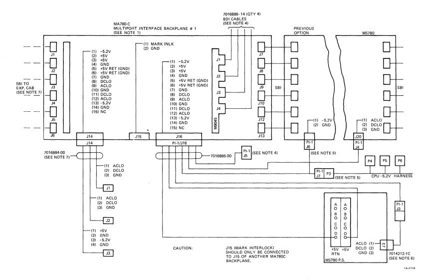
Figure 9-20 MA780C Power Cables with One Port
