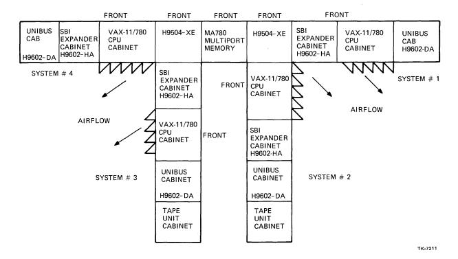
Figure 9-15 Four VAX-11/780 Systems in a "pi" Configuration
