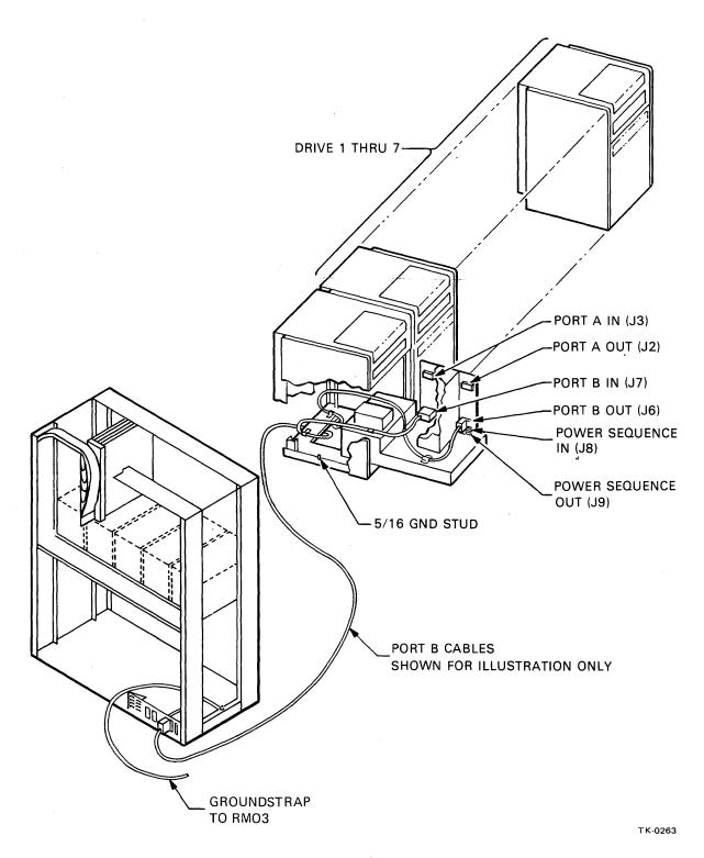
Figure 1-11 RM03 Cable Connections
