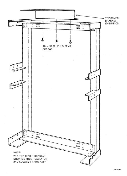
Figure 9-9 H9504-XE Top Cover Bracket Installation
