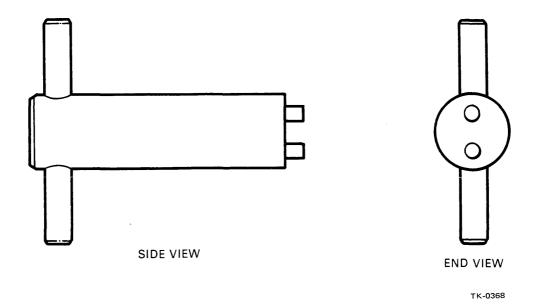
Figure 1-5 UNIBUS Expander Cabinet Opening Tool
