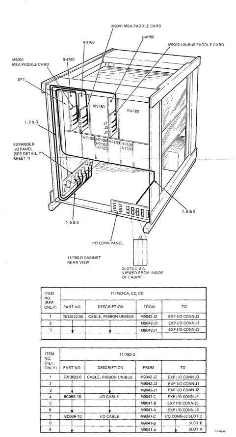
Figure 12-1 VAX-11/780 System Interconnect Diagram (Sheet 2 of 2)
