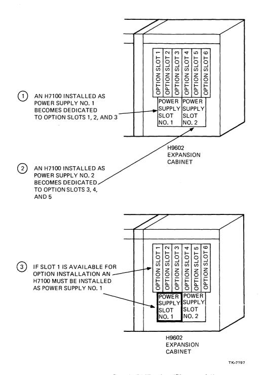
Figure 5-1 Power Supply Utilization (Sheet 1 of 2)
