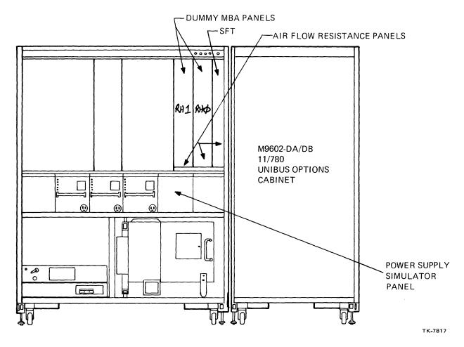
Figure 10-2 Standard VAX (SV-AXHHA) Cabinet Configuration (Front View)
