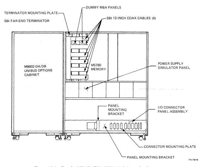
Figure 12-2 Standard VAX (SV-AXHHA) Cabinet Configuration
