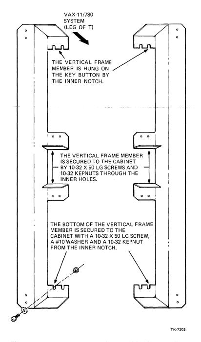
Figure 9-7 H9504-XE Vertical Frame Member Installation
