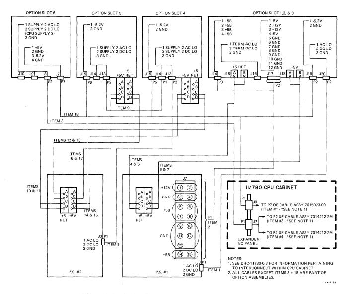
Figure 5-4 Option Power Supply Cabling (Sheet 2 of 3)
