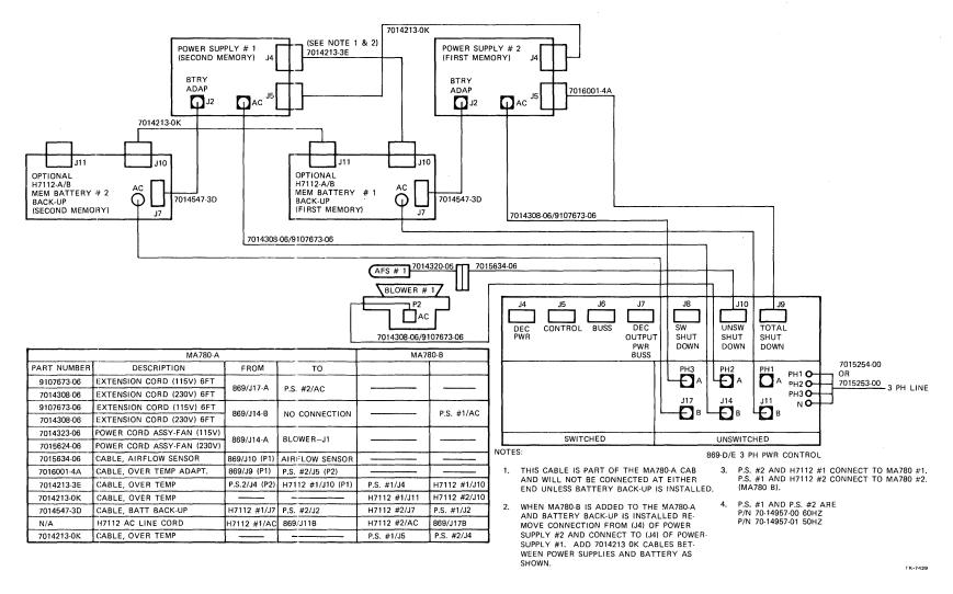
Figure 9-30 MA780B Option AC Power Connections
