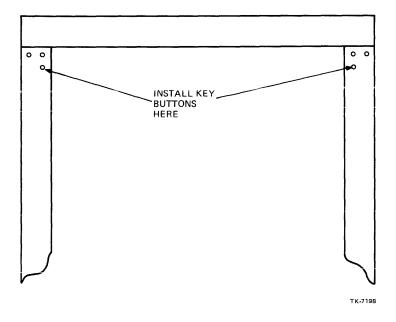
Figure 9-6 H9504-XE Key Button Installation
