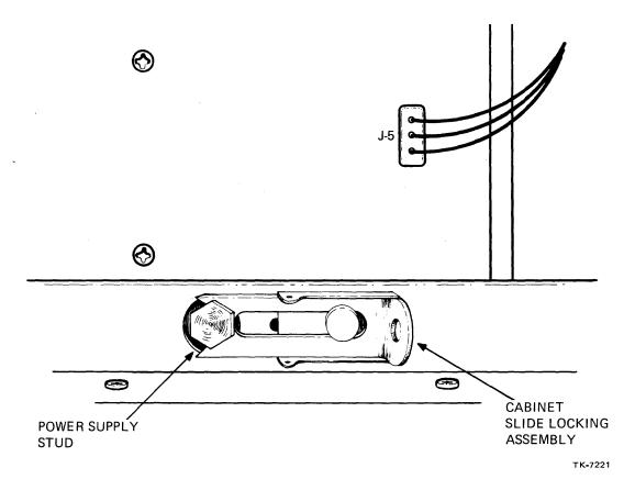
Figure 5-2 Power Supply Slidelock Details
