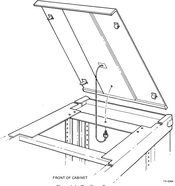
Figure 1-4 Top Cover Fastener
