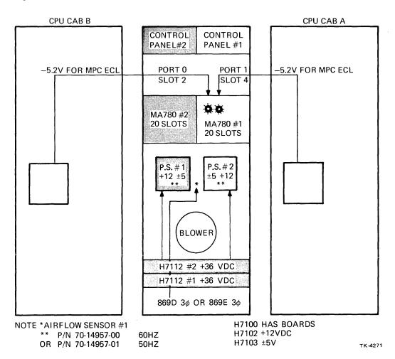
Figure 9-25 MA780A (#1) and MA780B (#2) Physical Location
