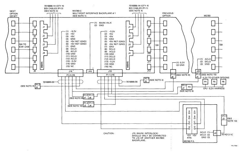
Figure 9-21 MA780C Power Cables with Two Ports
