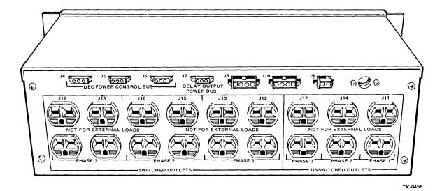
Figure 9-32 869E Power Controller (Front and Back Views)
