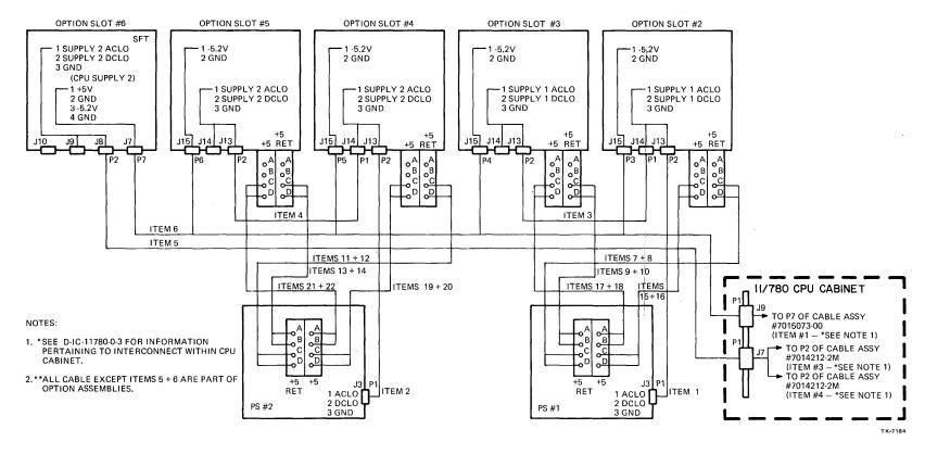
Figure 5-4 Option Power Supply Cabling (Sheet 1 of 3)
