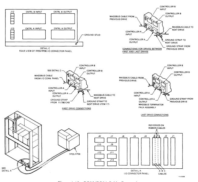
Figure 1-10 RP05/RP06 Cable Connections
