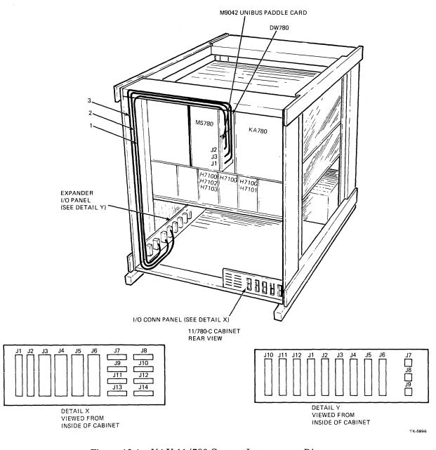
Figure 12-1 VAX-11/780 System Interconnect Diagram (Sheet 1 of 2)
