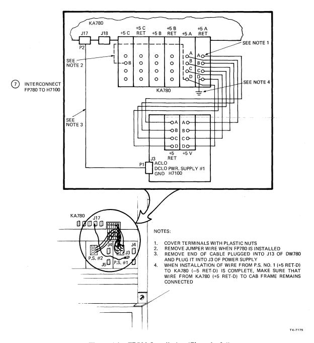
Figure 4-2 FP780 Installation (Sheet 3 of 4)
