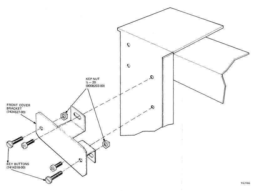
Figure 9-11 H9504-XE Front Cover Bracket Installation
