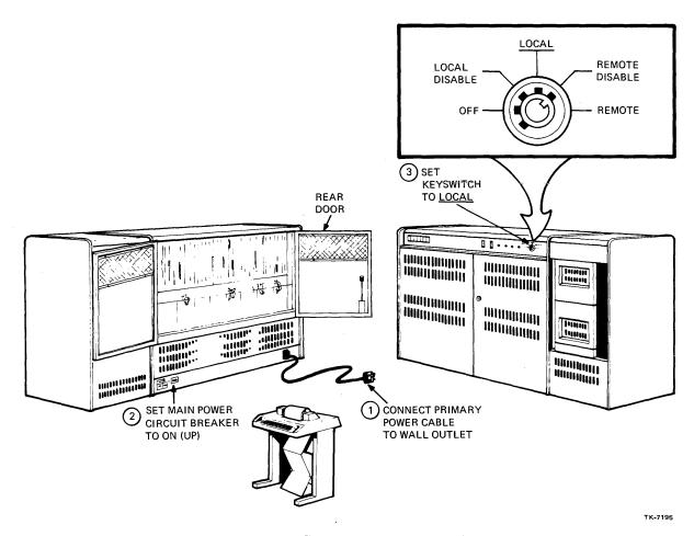
Figure 4-3 System Turn-On Procedure
