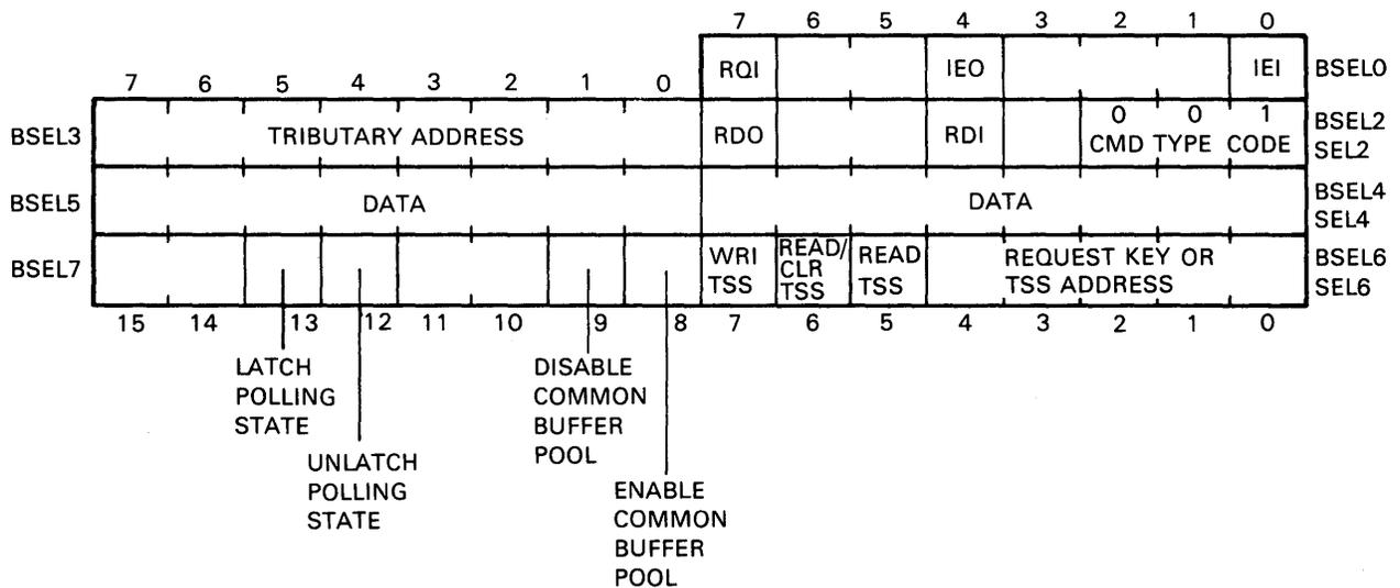
Figure 3-6 Control Command Format
