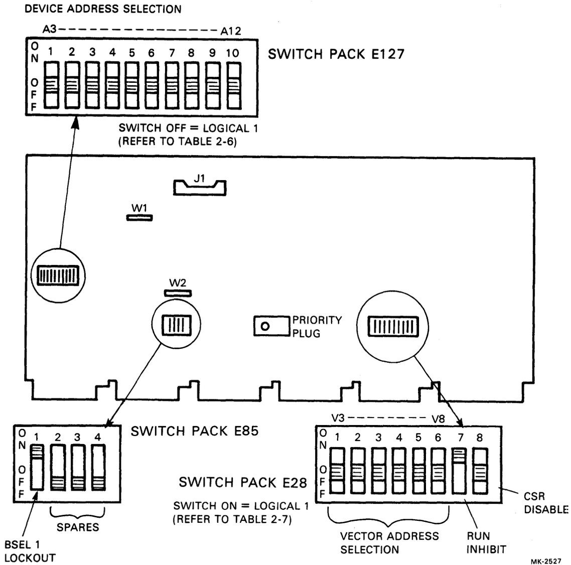
Figure 2-3 M8207-YA Microprocessor Switch/Jumper Locations
