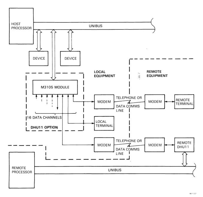
Figure 1-2 Example of DHU11 Configuration
