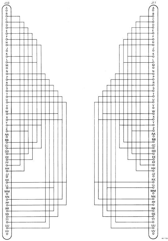
Figure 2-5 Staggered-Loopback Circuit of H3029
