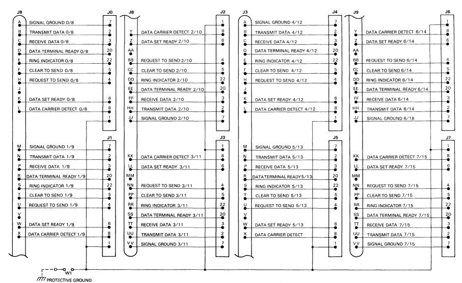
Figure 2-4 H3029 Circuit Diagram
