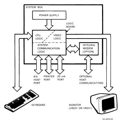
Figure 7-1 VT240-Series Terminal System Block Diagram
