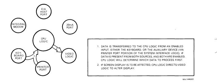
Figure 3-5 System Interaction in Local (Printer Port as Input Port)
