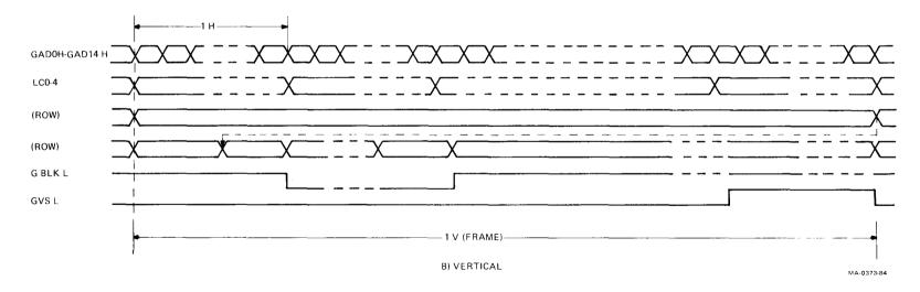
Figure 6-13 PD7220 GDC Timing Diagram: Video Sync Signals
