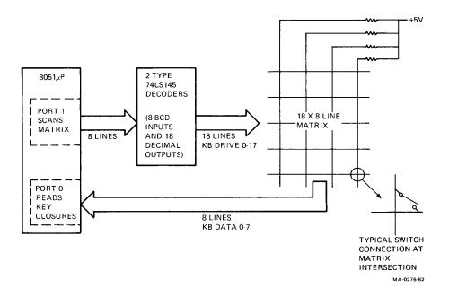
Figure 7-5 Matrix Scanning Block Diagram
