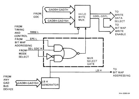
Figure 6-28 Hi/Lo Byte Select Block Diagram
