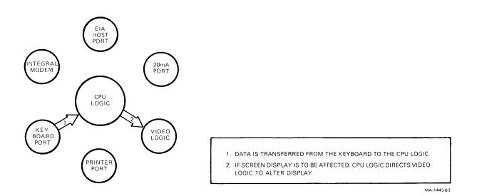
Figure 3-2 System Interaction in Set-Up
