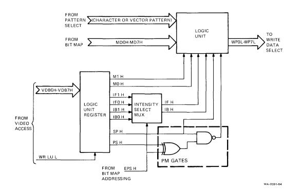
Figure 6-31 Logic Unit Block Diagram
