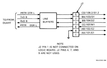
Figure 5-9 Printer Interface (I/F) Block Diagram
