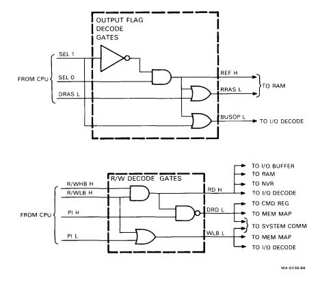
Figure 4-12 Control Gates Block Diagram
