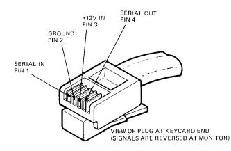
CABLE CONNECTOR WIRING
