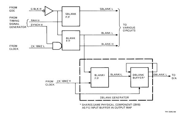
Figure 6-22 BLANK Generator Block Diagram
