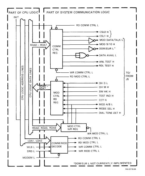
Figure 5-7 Communication/Modem (Comm/Modem) Control Block Diagram
