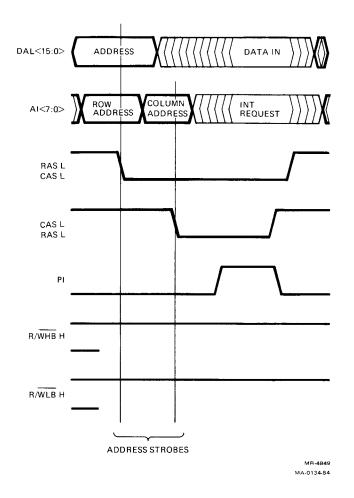
Figure 4-7 Tll 16-Bit Dynamic Read Transaction Diagram
