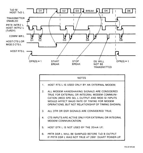
Figure 5-5 2681 DUART: Transmit Data Timing Diagram
