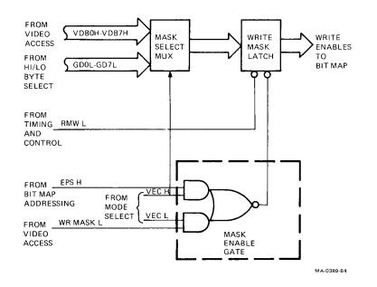
Figure 6-29 Bit Map Write Enable Block Diagram
