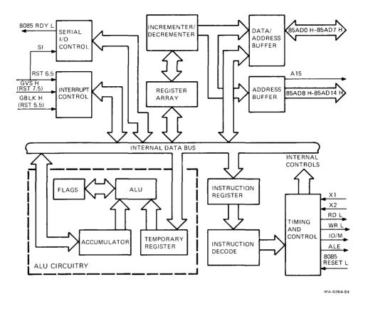
Figure 6-4 8085A-2 Microprocessor Device Internal Block Diagram
