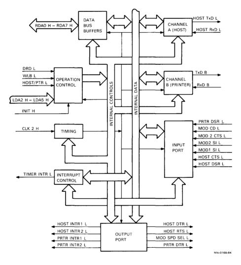
Figure 5-4 2681 DUART Internal Circuits Block Diagram
