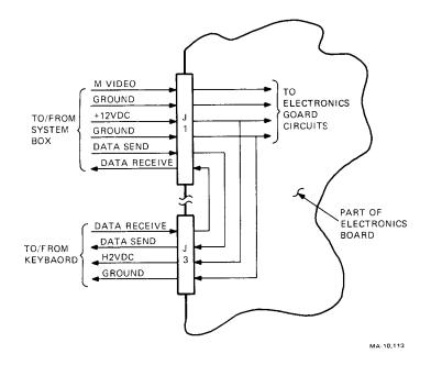
Figure 8-4 Monochrome Monitor System Communications Diagram
