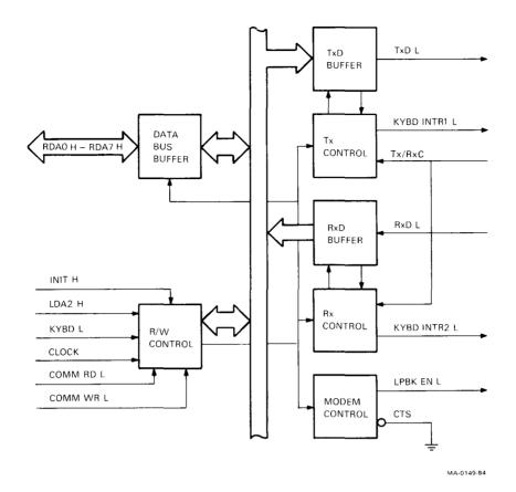
Figure 4-24 8251A USART Internal Circuits Block Diagram
