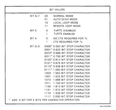
Figure D-5 2681 DUART: Mode Register 2 (MR2) (Channel A and B)
