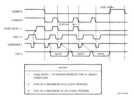
Figure 4-25 8251A USART Transmit Data (TxD) Timing Diagram
