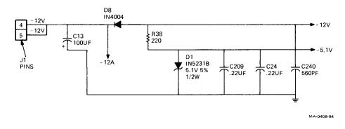
Figure 9-13 -12 V Input Circuit
