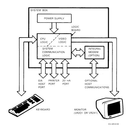
Figure 3-1 VT240 Series Terminal System Block Diagram
