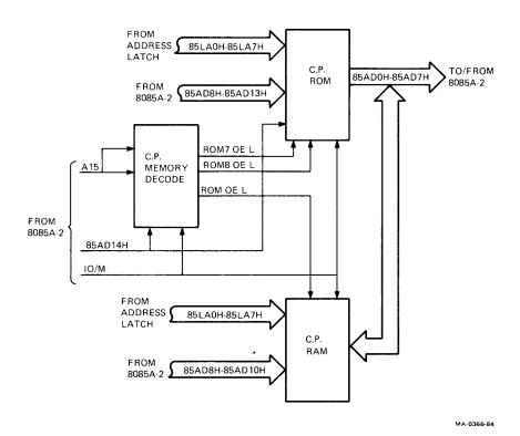
Figure 6-6 Character Processor (CP) Memory Block Diagram  Character Processor (CP) Memory Decode -- decodes Al5 and 85AD14 H inputs into either a ROM (ROM7 OE or ROM8 OE) or RAM (RAM OE) enable signal, when memory is to be accessed (IO/M low).
