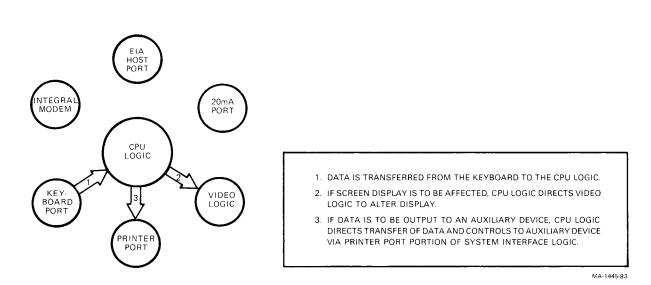
Figure 3-4 System Interaction in Local (Printer Port as Output Port)
