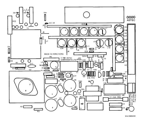
Figure 9-9 PS1 Component Layout
