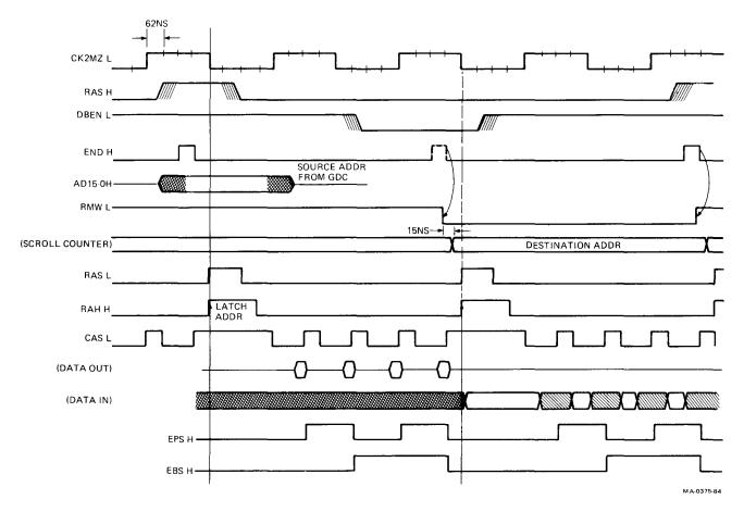
Figure 6-15 PD722Ø GDC Timing Diagram: Video DMA Write Transaction
