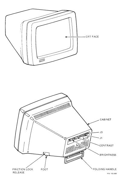
Figure 8-2 Monochrome Monitor Exterior View
