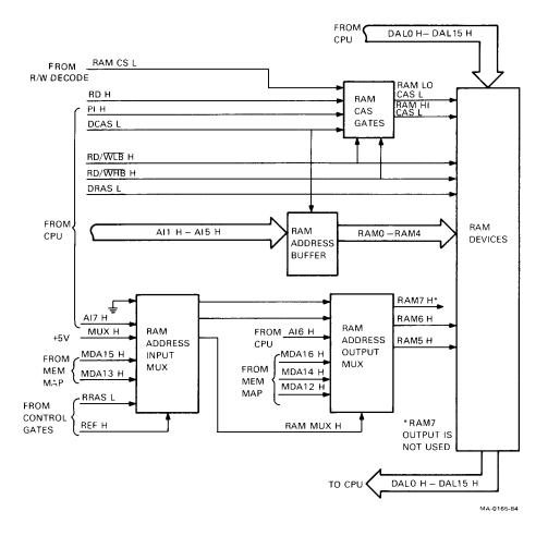
Figure 4-18 Random Access Memory (RAM) Block Diagram
