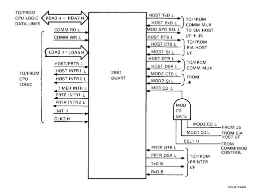
Figure 5-3 DUART Block Diagram
