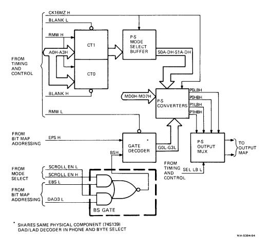
Figure 6-34 Parallel-to-Serial (P/S) Converter Block Diagram
