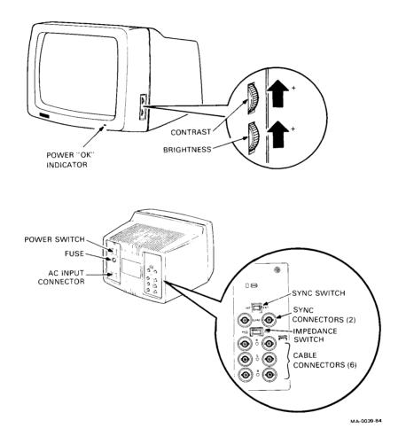
Figure 2-3 VR241 Monitor Controls, Indicators, and Connectors (Front and Rear)
