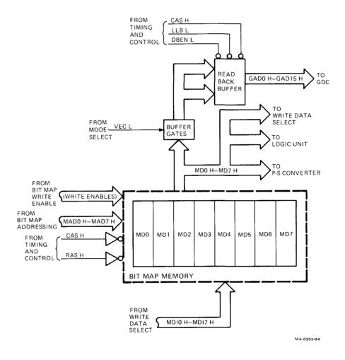
Figure 6-33 Bit Map Block Diagram
