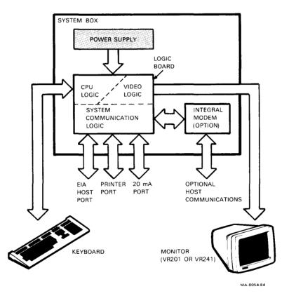
Figure 9-1 VT24Ø-Series Terminal System Block Diagram
