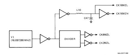
Figure 6-17 Clock Generator Block Diagram
