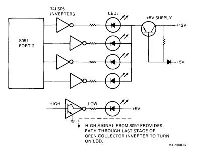
Figure 7-9 Indicator (LED) Control Circuit
