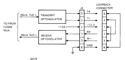
VOLTAGE POTENTIALS FOR LOOPBACK TEST; PINS 4 AND 6 ARE NOT USED AT J4 OR AT LOOPBACK CONNECTOR.
