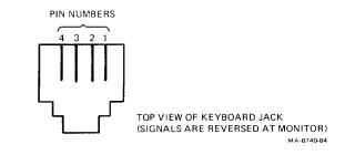
Figure 2-9 Connector for BCC01 Cable
