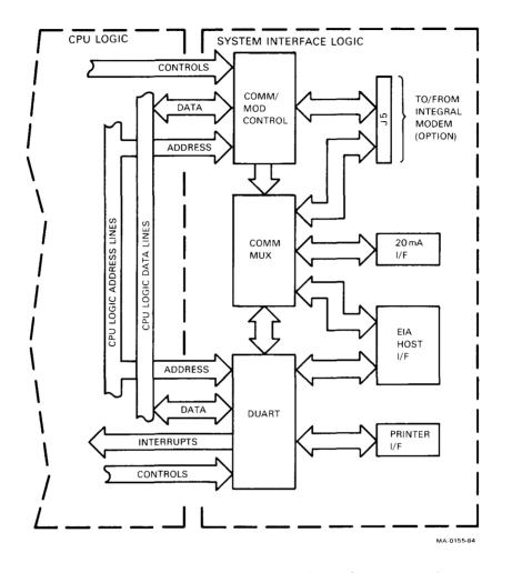
Figure 5-2 System Communications Logic Block Diagram
