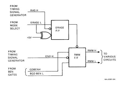
Figure 6-21 Read-Modify-Write (RMW) Generator Block Diagram
