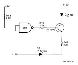
Figure 9-14 DC Power OK Circuit
