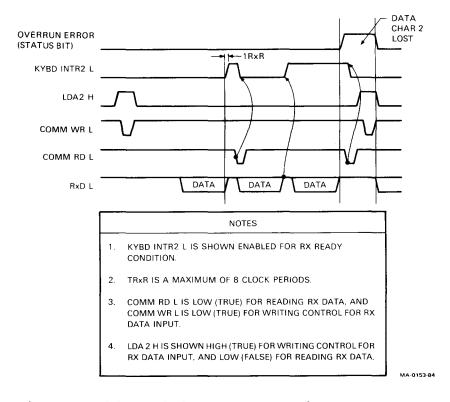
Figure 4-26 8251A USART Receive Data (RxD) Timing Diagram
