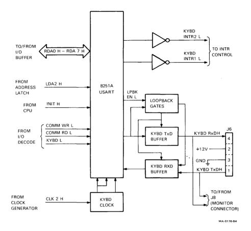
Figure 4-23 Keyboard Interface (I/F) Block Diagram
