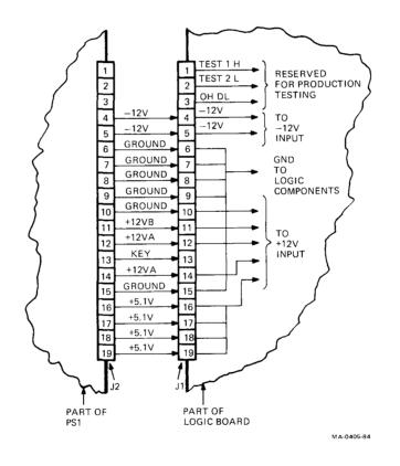
Figure 9-10 Logic Board DC Power Input Connector
