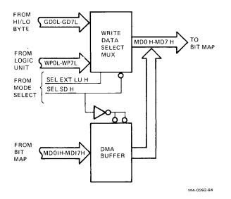
Figure 6-32 Write Data Select Block Diagram
