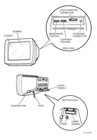
Figure 2-2 VR201 Monitor Controls, Indicators, and Connectors
