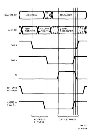
Figure 4-8 Tll 16-Bit Dynamic Write Transaction Diagram
