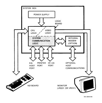
Figure 5-1 VT24Ø-Series Terminal System Block Diagram
