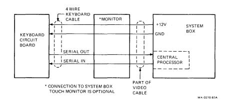
Figure 7-3 Keyboard Cable Connections
