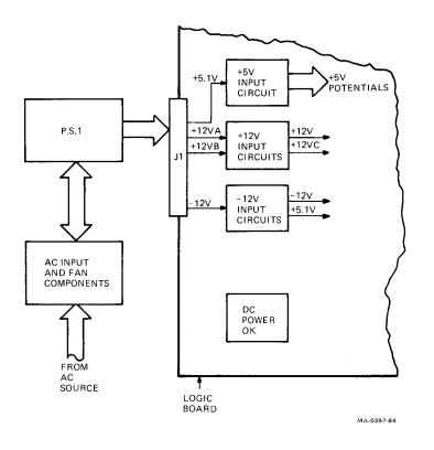
Figure 9-2 Power Supply Block Diagram
