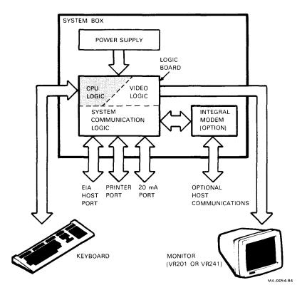
Figure 4-1 VT24Ø-Series Terminal System Block Diagram
