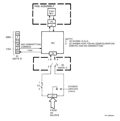
Figure 9-3 AC Input and Fan Components Block Diagram
