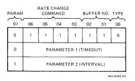
Figure 7-17 Change Rates in Buffer 3 Example
