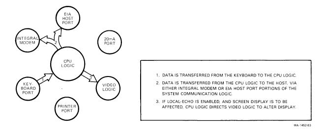
Figure 3-11 System Interaction in On-Line (Printer Port as Inactive or Output Port)
