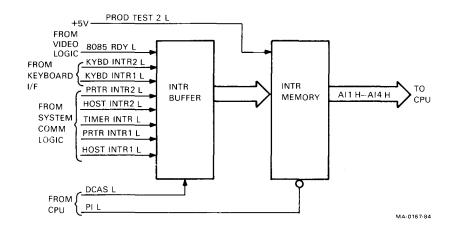
Figure 4-28 Interrupt Control Block Diagram
