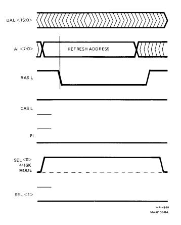
Figure 4-9 Tll Refresh Transaction Diagram
