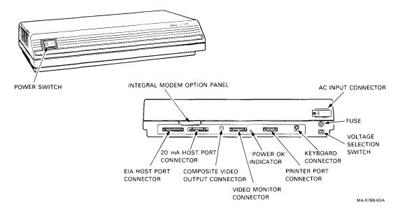
Figure 2-1 System Box Controls, Indicators, and Connectors
