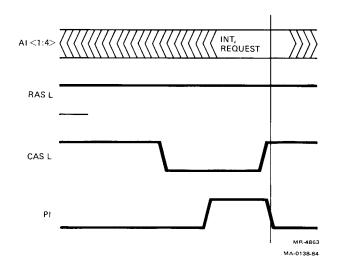
Figure 4-10 Tll ASPI Transaction Diagram
