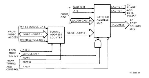
Figure 6-26 Address Select Block Diagram
