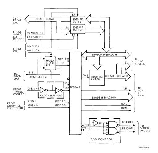
Figure 6-3 Character Processor (CP) Block Diagram
