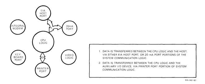
Figure 3-10 System Interaction in On-Line (Printer Port as I/O Port)
