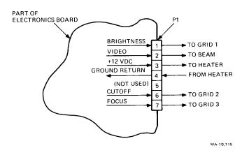
Figure 8-8 Monitor Module Pl Pinout
