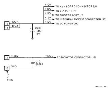
Figure 9-12 +12 V Input Circuit
