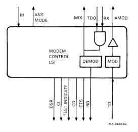
Figure 10-10 Modem Control LSI
