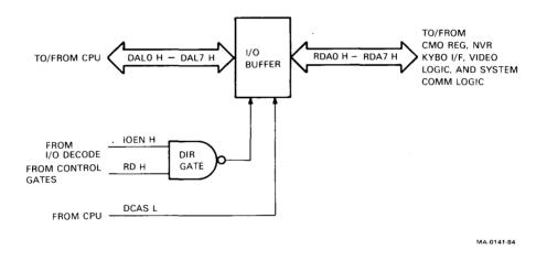
Figure 4-21 I/O Buffer Block Diagram
