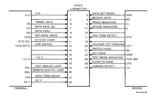
Figure 10-11 Stack Connector
