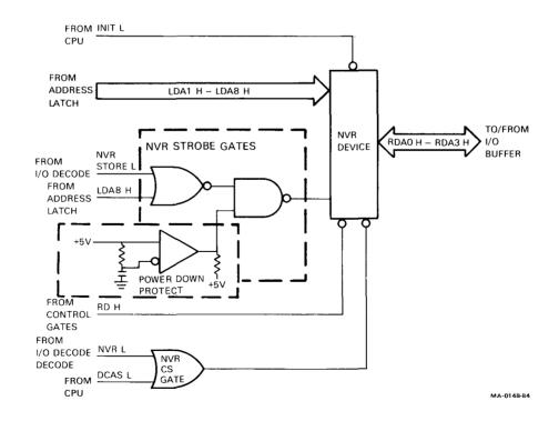
Figure 4-27 Nonvolatile RAM (NVR) Block Diagram
