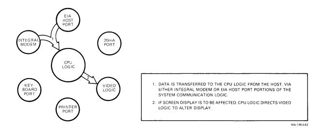
Figure 3-12 System Interaction in On-Line (Printer Port as Inactive or Input Port)
