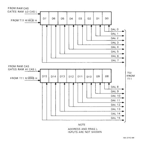
Figure 4-20 RAM Devices Array
