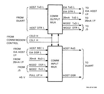
Figure 5-8 Comm Mux Block Diagram
