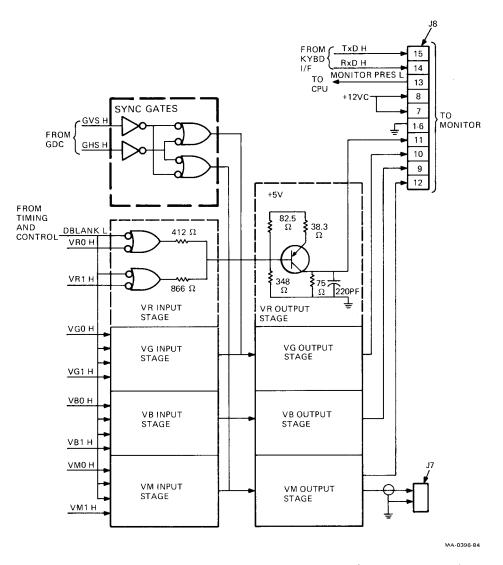
Figure 6-36 Digital-to-Analog (D/A) Block Diagram
