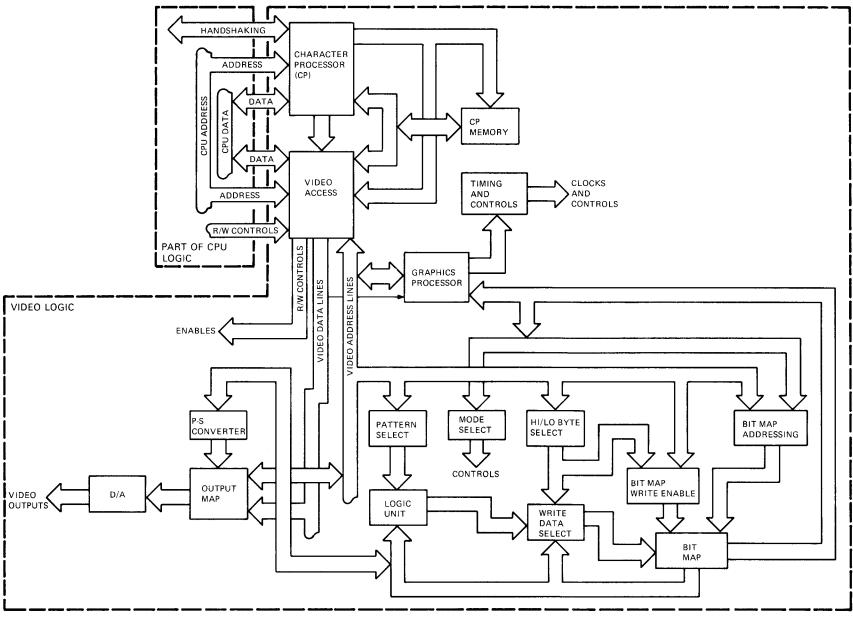
Figure 6-2 Video Logic Block Diagram
