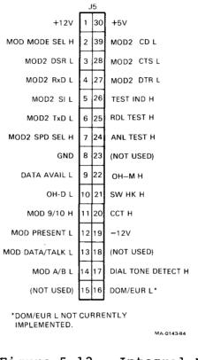
Figure 5-12 Integral Modem Option Connector (J5) Pinout
