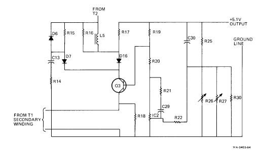
Figure 9-8 +5.1 V Crowbar Circuit
