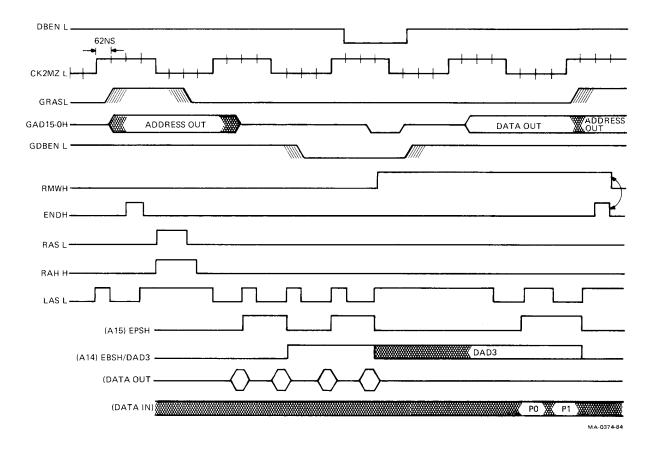
Figure 6-14 PD7220 GDC Timing Diagram: 2-Plane Write Transaction
