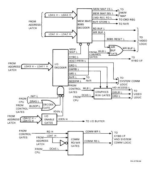
Figure 4-22 I/O Decode Block Diagram
