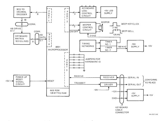
Figure 7-4 LK201 Keyboard Block Diagram
