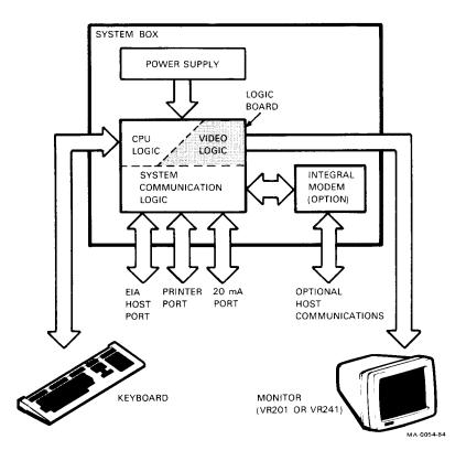
Figure 6-1 VT24Ø-Series Terminal System Block Diagram
