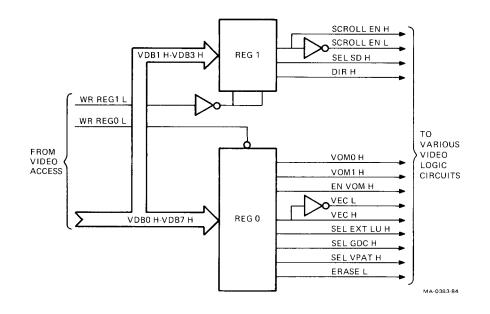
Figure 6-23 Mode Select Block Diagram
