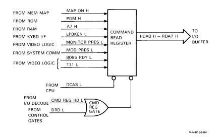
Figure 4-29 Command Register Block Diagram
