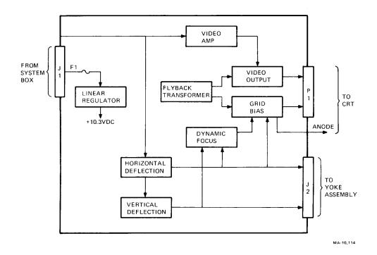
Figure 8-7 Monitor Module Block Diagram
