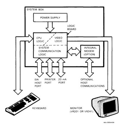
Figure 8-1 VT24Ø-Series Terminal System Block Diagram
