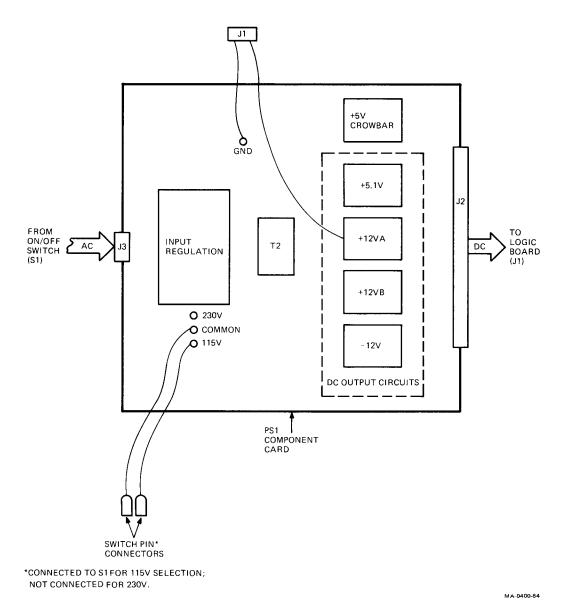
Figure 9-5 Power Supply 1 (PS1) Block Diagram
