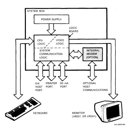
Figure 10-1 VT240-Series Terminal Block Diagram
