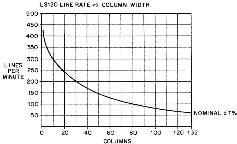
Figure 4-2 LS120 Line Rate Versus Column Width
