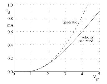
effect can be observed in Figure 16 which plots  $I_d$  vs  $V_{gs}$  for  $V_{ds} = 5$ . While the
