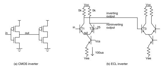
Figure 32: CMOS and ECL Test Circuits
