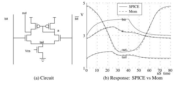
Figure 73: Sense Amplifier for Static RAM.
