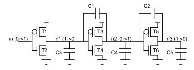
Figure 69: Clusters Coupled by Floating Capacitors.
