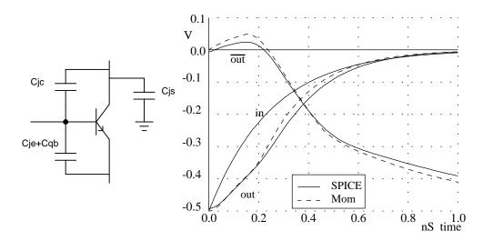
Figure 34: Level-1 Bipolar Model has Floating Capacitors.
