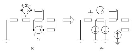
Figure 66: Branch Tearing of Nearly Leaky Tree.
