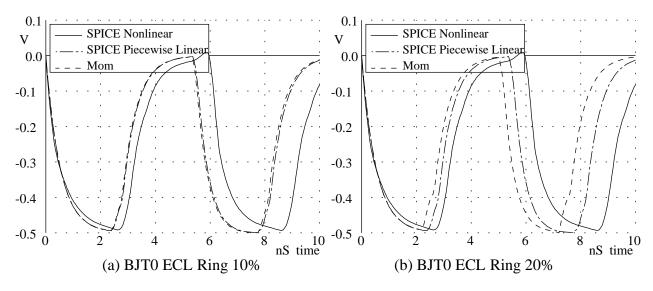
Figure 43: ECL Level-0 Ring: SPICE vs PWL vs Mom.
