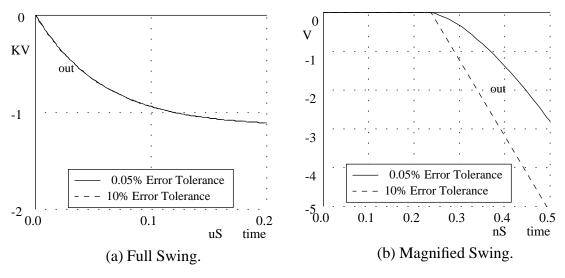
Figure 40: Large Signal Swing for CMOS NAND Gate.
