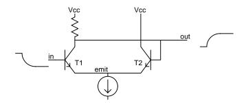
Figure 38: Schmitt Trigger
