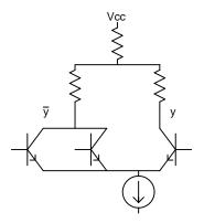
Figure 77: Resistor Tee as ECL Load.
