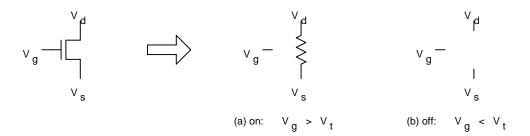
Figure 12: Switched Resistor Model.
