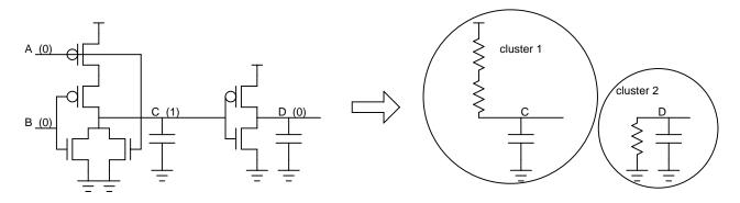
Figure 9: Decomposition of Circuit into Clusters.
