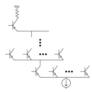
Figure 76: ECL Current Steering Networks.
