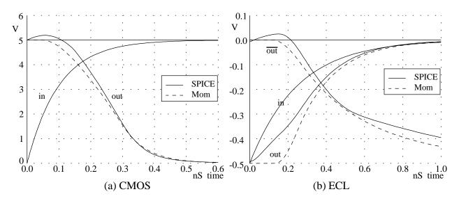
Figure 33: Grounded Capacitor Approximations.
