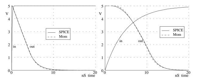
Figure 23: Inverters Using Piecewise Linear vs SPICE Transistors.
