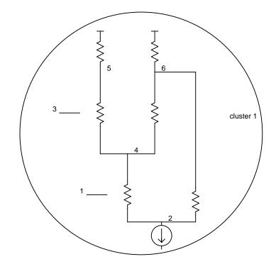
Figure 60: Resistor Model for Bipolar Transistor Results in Loops in ECL Gates
