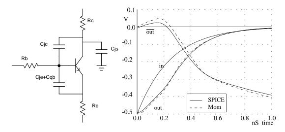
Figure 35: Level-2 Bipolar Model has Floating Capacitors and Parasitic Resistors
