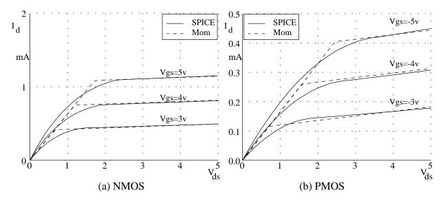
Figure 21: Piecewise Linear vs SPICE I-V Characteristics: SPICE Level-3 models for MOSIS  $1.2\mu$  Process.
