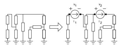
Figure 63: Circuit Partitioning via Branch Tearing.
