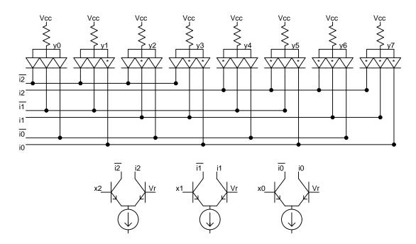
Figure 78: Diode Decoder.
