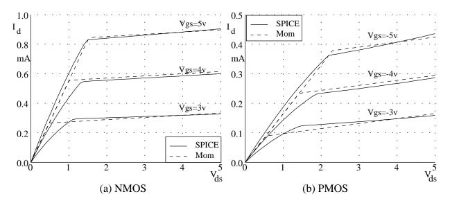
Figure 20: Piecewise Linear vs SPICE I-V Characteristics:  $V_{gs} = 3,4$ , and 5 volts, SPICE Level-2 models for MOSIS  $2\mu$  Process.
