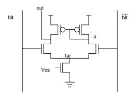
Figure 27: SRAM Sense Amplifier
