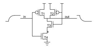
Figure 39: 2 Input CMOS NAND Gate.
