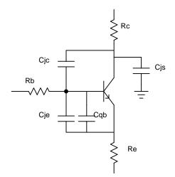
Figure 94: Nonlinear Capacitances in SPICE bjt model
