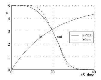
Figure 25: Slow Input to CMOS Gate Accentuates Modeling Errors.
