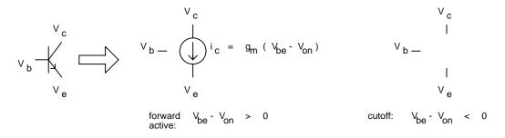
Figure 29: Piecewise Linear Bipolar Model.
