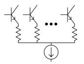
Figure 80: Emitter Degeneration Resistors to Cause Current Sharing.
