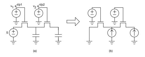
Figure 52: Transistor-capacitor tree.
