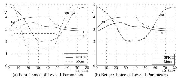
Figure 28: Simulated Response of SRAM Sense Amplifier.
