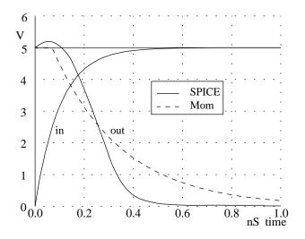
Figure 14: Response of Level-0 Inverter Compared to SPICE.
