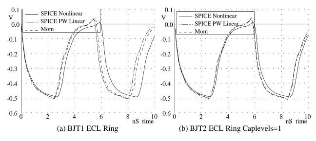
Figure 44: ECL Level-1 & -2 Rings: SPICE vs PWL vs Mom.
