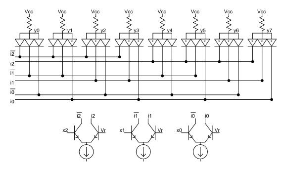
Figure 62: Diode Decoder.
