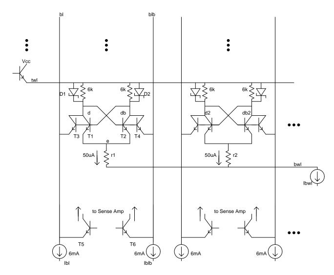
Figure 81: Schottky Clamped ECL RAM.
