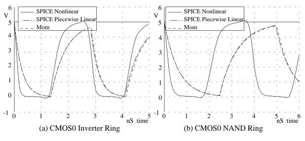
Figure 41: CMOS Level-0 Ring: SPICE vs PWL vs Mom.
