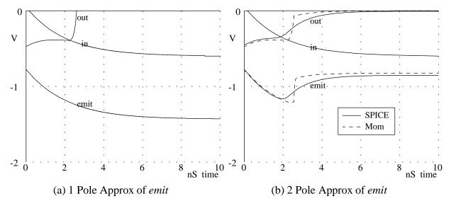
Figure 45: Simulation of Schmitt Trigger
