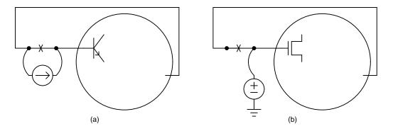
Figure 68: Tearing of feedback.
