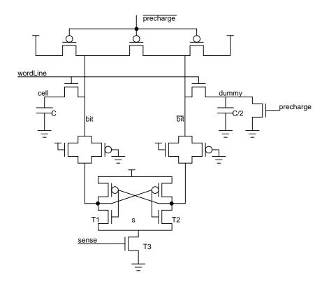
Figure 74: Dynamic RAM Cell and Sense Amplifier
