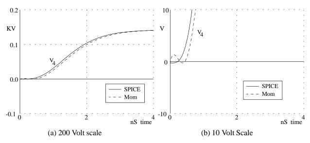
Figure 48: Initial Segment in the Response of ECL Cascade.
