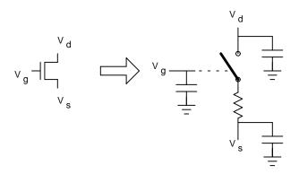
Figure 8: Switched Resistor Model
