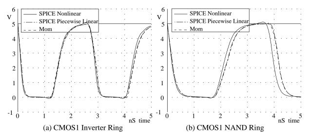
Figure 42: CMOS Level-1 Ring: SPICE vs PWL vs Mom.
