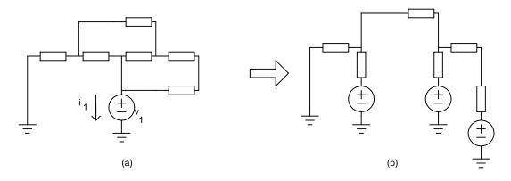
Figure 67: Node Tearing of Nearly Leaky Tree.
