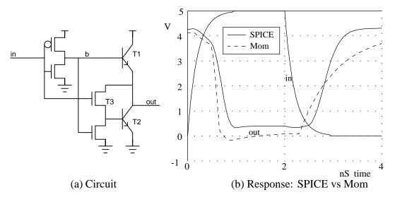
Figure 84 (a) shows one of several variations of the BiCMOS buffer[GM88]. In general,
