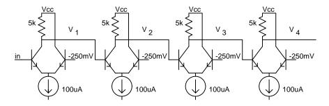
Figure 47: Cascade of ECL Inverters
