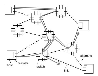
Figure 1: A Portion of an Autonet Installation
