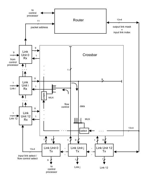
Figure 2: Structure of an Autonet Switch
