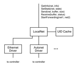
Figure 4: Structure of Low-level LAN Software for the Firefly
