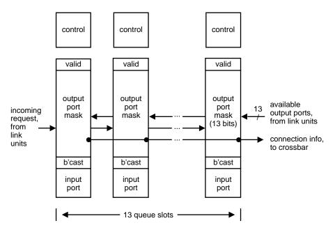
Figure 7: Scheduling Engine for Switch Output Ports
