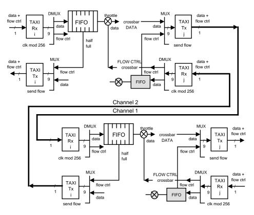
Figure 5: Switch-to-switch Flow Control Mechanism
