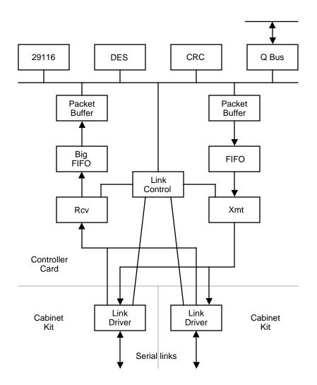
Figure 3: Structure of the Q-bus Autonet Controller
