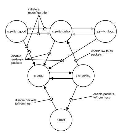
Figure 8: Switch Port States and Transitions
