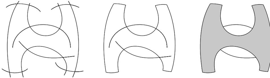
Figure 9: Cleaning a face removes its dangling edges.
