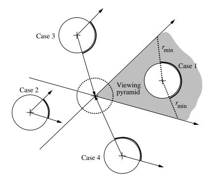
Figure 4: Different cases for forward mapping (top view).
