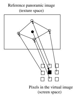
Figure 5: Geometric interpolation for filling in holes left by forward mapping.
