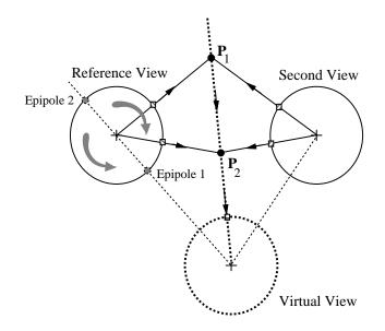
Figure 3: Handling occlusion using back-to-front ordering (top view).
