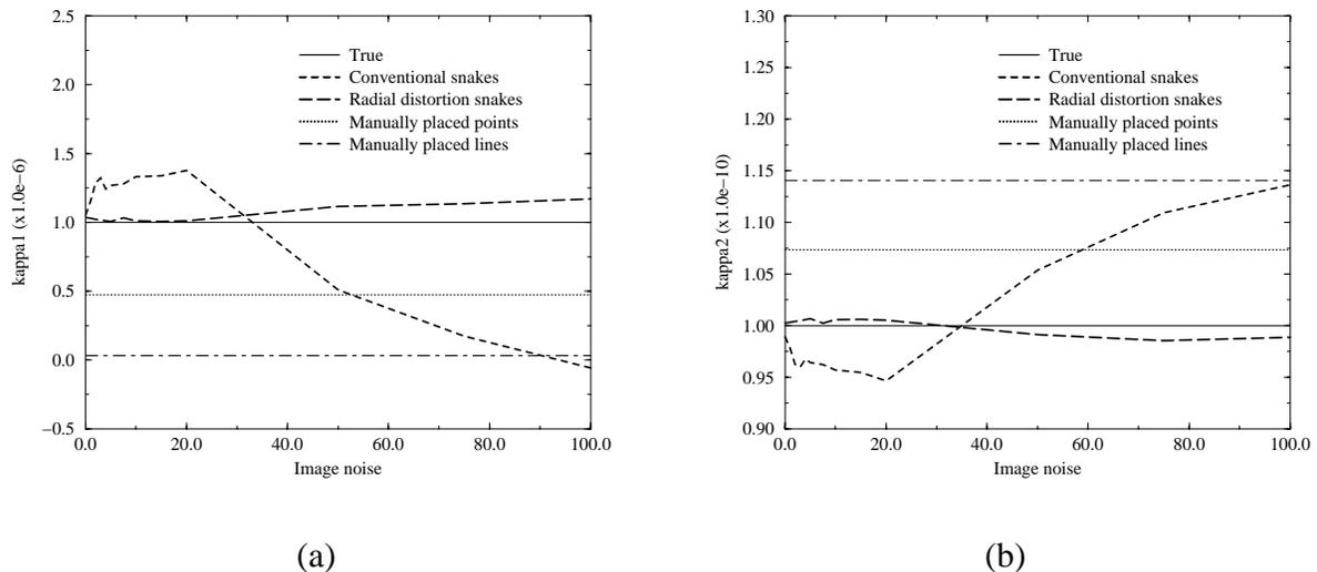
Figure 3: Graphs showing the effect of gaussian image noise (standard deviation in intensity level) on recovered radial distortion parameters: (a)  $\kappa_1$  (true value is  $10^{-6}$ ), and (b)  $\kappa_2$  (true value is  $10^{-10}$ ). Note that for the manual method, the points were placed on the image with no noise. Also, for the other two methods, the snakes were initialized on the image with no noise.
