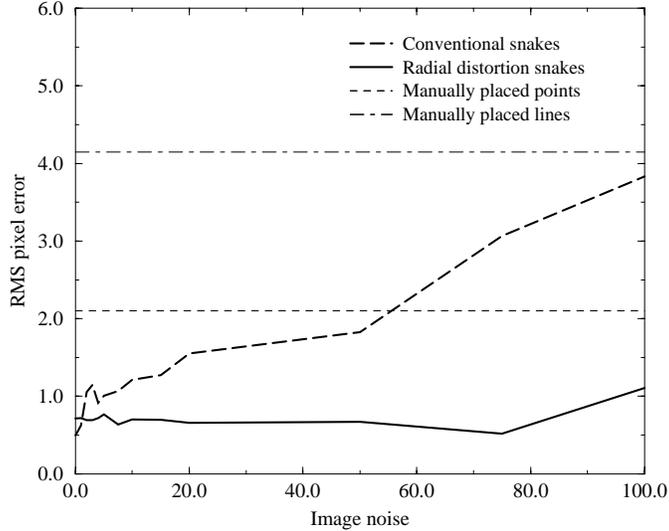
Figure 4: Graph showing the effect of gaussian image noise (standard deviation in intensity level) on RMS undistortion error  $E_{RMS}$ .
