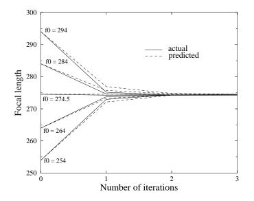
Figure 6: Graph of estimated focal length vs. number of iteration. f0 is the initial estimated focal length; the actual focal length is 274.5. The solid lines represent actual values whereas dashed lines represent predicted values.
