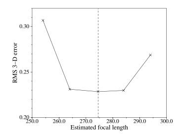
Figure 17: Graph of RMS 3D error of recovered stereo data vs. estimated focal length. The true focal length is 274.5 (indicated by the vertical dashed line).
