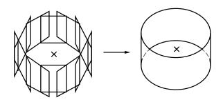
Figure 1: Compositing multiple rotated camera views into a panorama. The ' $\times$ ' marks indicate the locations of the camera optical and rotation center.
