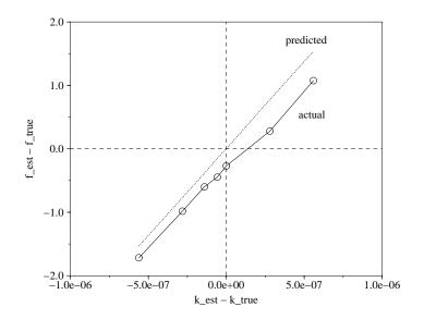
Figure 12: Graph of equivalent focal length error vs. error in  $\kappa$ , the radial distortion factor. The true focal length ( $f_{true}$ ) is 274.5 and the true radial distortion factor ( $\kappa_{true}$ ) is  $2.8 \times 10^{-7}$ .
