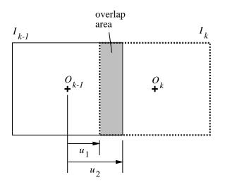
Figure 5: Overlap between successive images  $I_{k-1}$  and  $I_k$ , with centers at  $O_{k-1}$  and  $O_k$  respectively.
