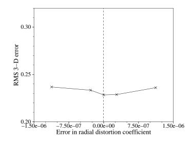
Figure 18: Graph of RMS 3D error of recovered stereo data vs. error in radial distortion coefficient  $\kappa$ . Typical real values of  $\kappa$  is of the order of  $10^{-7}$ . The zero error in  $\kappa$  is indicated by the vertical dashed line.
