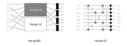
Figure 3: A MERGER [8] balancing network.
