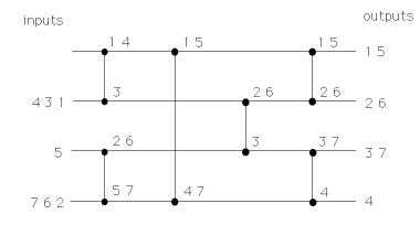
Figure 2: A sequential execution for a COUNTER[4] counting network.
